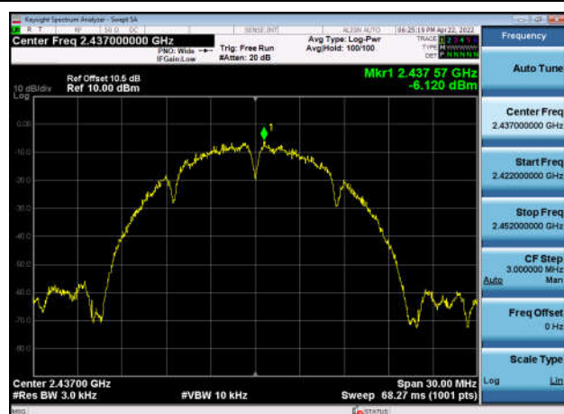
Power spectral density-802.11g ,2412MHz,Ant0
