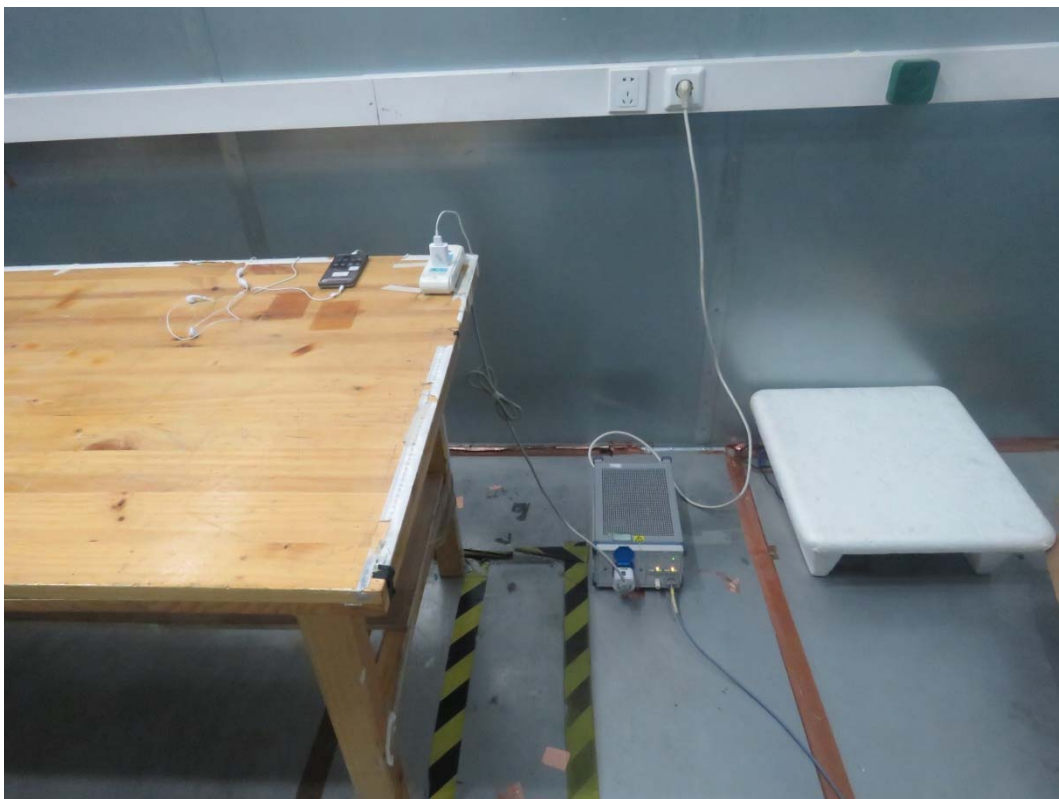
Picture 2 Conducted Emission Test Setup
