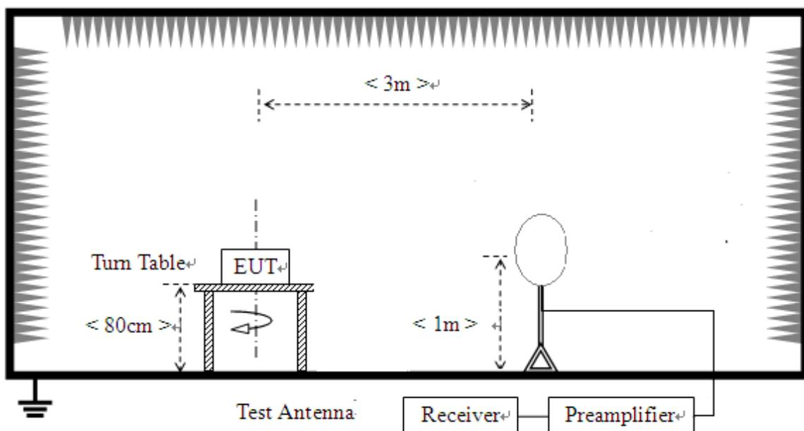
**For radiated emissions from 30MHz to 1GHz**
