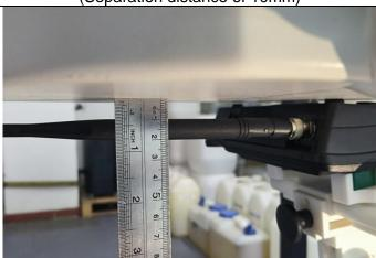
Back Side and Ant Vertical (Separation distance of 10mm)
