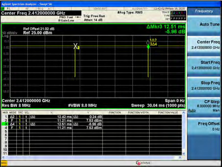
Duty cycle plot (802.11b(1Mbps))
