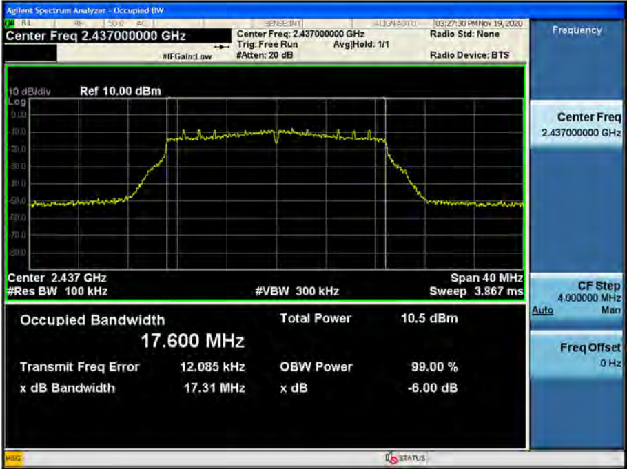
6dB Bandwidth plot (802.11n_HT20-CH 6)
