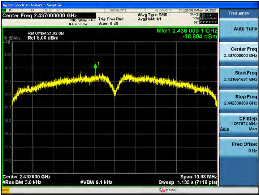
Power Spectral Density (802.11b-CH 6)
