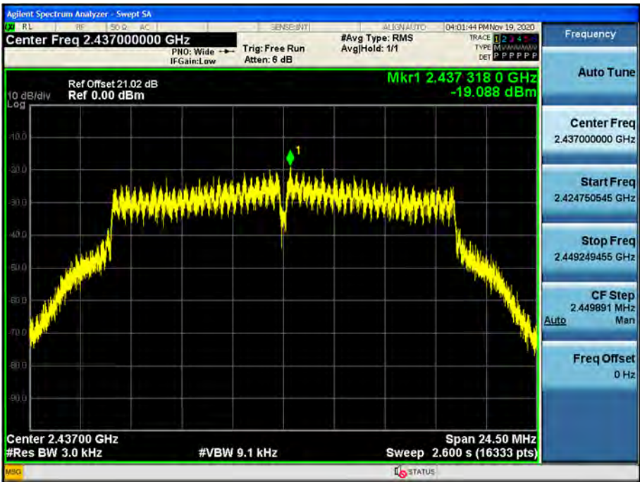
Power Spectral Density (802.11g-CH 6)
