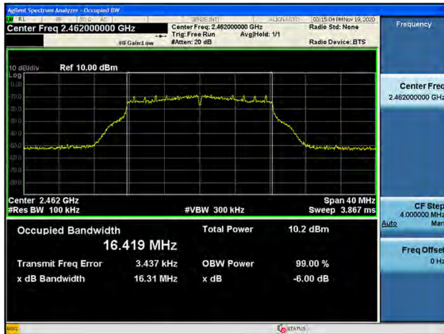
6dB Bandwidth plot (802.11g-CH 11)
