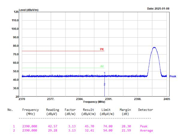
Project No.: 2403A43118E-RF Tester: coco Tian Condition: PK trace RBW:1MHz; VBW:3MHz; SWT:0.3sec Polarization: Vertical Note: 3EDR Low Channel 2402MHz Chain 0
