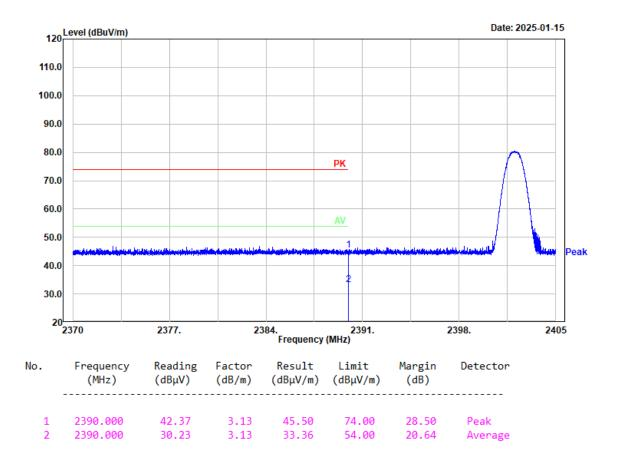
Project No.: 2403A43118E-RF Tester: coco Tian Condition: PK trace RBW:1MHz; VBW:3MHz; SWT:0.3sec Polarization: Vertical Note: BDR Low Channel 2402MHz Chain 1
