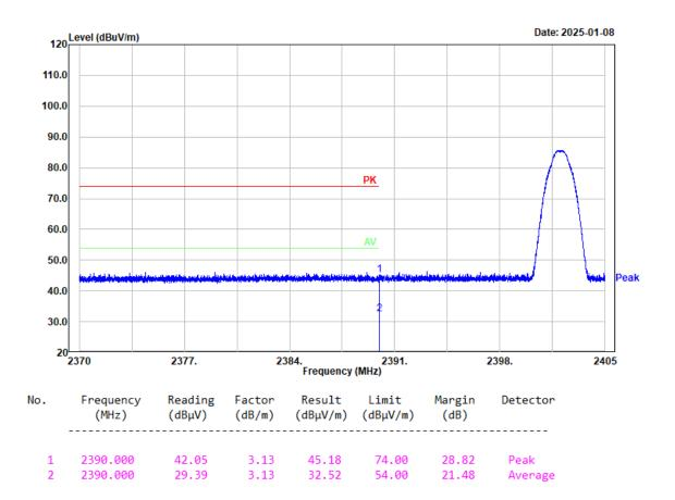
Project No.: 2403A43118E-RF Tester: coco Tian Condition: PK trace RBW:1MHz; VBW:3MHz; SWT:0.3sec Polarization: Horizontal Note: 2EDR High Channel 2480MHz Chain 0
