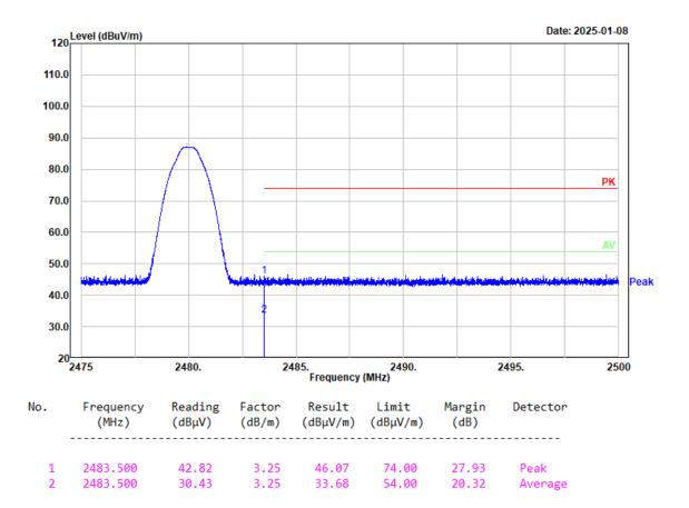
Project No.: 2403A43118E-RF Tester: coco Tian Condition: PK trace RBW:1MHz; VBW:3MHz; SWT:0.3sec Polarization: Horizontal Note: 3EDR Low Channel 2402MHz Chain 0
