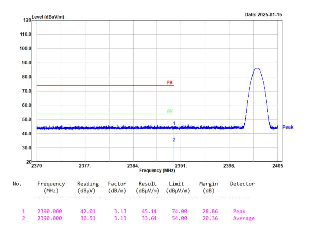
Project No.: 2403A43118E-RF Tester: coco Tian Condition: PK trace RBW:1MHz; VBW:3MHz; SWT:0.3sec Polarization: Horizontal Note: 3EDR High Channel 2480MHz Chain 1
