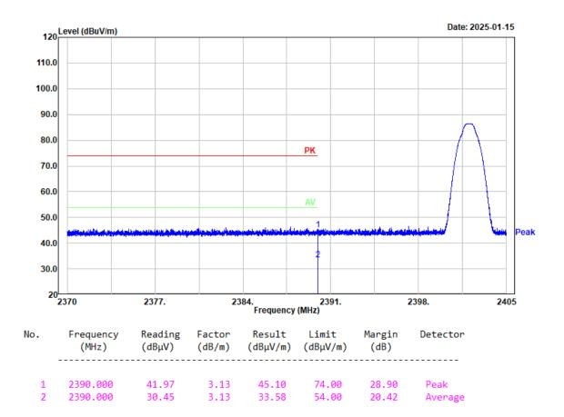
Project No.: 2403A43118E-RF Tester: coco Tian Condition: PK trace RBW:1MHz; VBW:3MHz; SWT:0.3sec Polarization: Horizontal Note: 2EDR High Channel 2480MHz Chain 1
