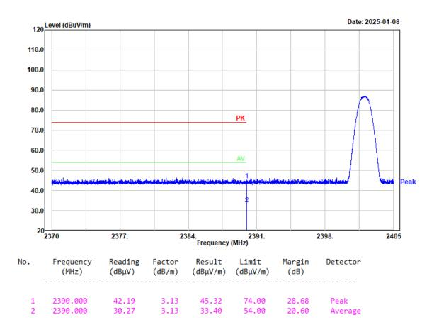
Project No.: 2403A43118E-RF Tester: coco Tian Condition: PK trace RBW:1MHz; VBW:3MHz; SWT:0.3sec Polarization: Horizontal Note: BDR High Channel 2480MHz Chain 0
