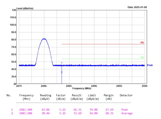
Project No.: 2403A43118E-RF Tester: coco Tian Condition: PK trace RBW:1MHz; VBW:3MHz; SWT:0.3sec Polarization: Vertical Note: BDR High Channel 2480MHz Chain 0
