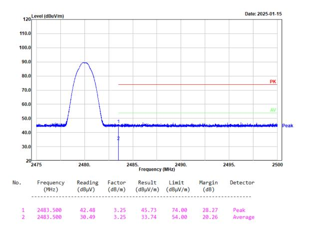
Project No.: 2403A43118E-RF Tester: coco Tian Condition: PK trace RBW:1MHz; VBW:3MHz; SWT:0.3sec Polarization: Horizontal Note: 3EDR Low Channel 2402MHz Chain 1
