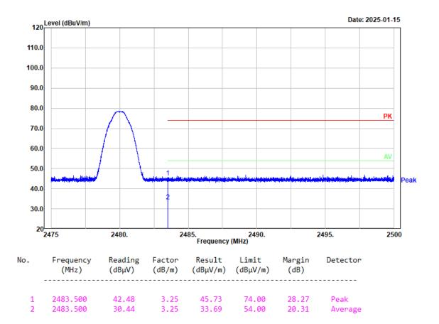
Project No.: 2403A43118E-RF Tester: coco Tian Condition: PK trace RBW:1MHz; VBW:3MHz; SWT:0.3sec Polarization: Vertical Note: 2EDR High Channel 2480MHz Chain 1
