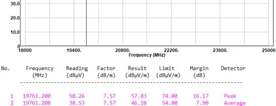
Project No.: 2403A43118E-RF Tester: coco Tian Condition: PK trace RBW:1MHz; VBW:3MHz; SWT:0.3sec Polarization: horizontal Note: 2EDR High Channel 2480MHz Chain 1
