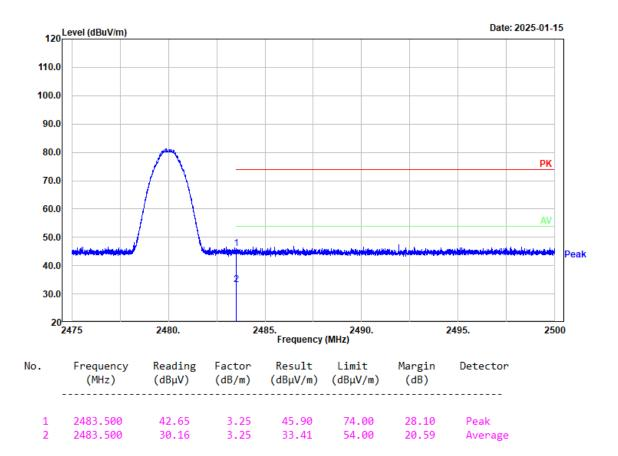
Project No.: 2403A43118E-RF Tester: coco Tian Condition: PK trace RBW:1MHz; VBW:3MHz; SWT:0.3sec Polarization: Vertical Note: 3EDR High Channel 2480MHz Chain 1
