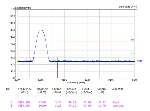
Project No.: 2403A43118E-RF Tester: coco Tian Condition: PK trace RBW:1MHz; VBW:3MHz; SWT:0.3sec Polarization: Horizontal Note: 2EDR Low Channel 2402MHz Chain 1
