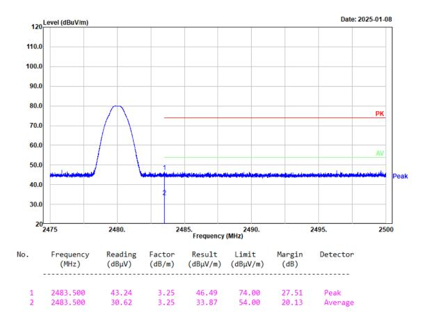
Project No.: 2403A43118E-RF Tester: coco Tian Condition: PK trace RBW:1MHz; VBW:3MHz; SWT:0.3sec Polarization: Vertical Note: 2EDR High Channel 2480MHz Chain 0
