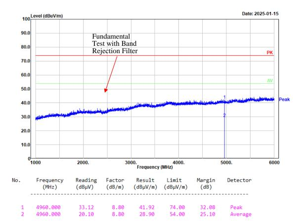
Project No.: 2403A43118E-RF Tester: coco Tian Condition: PK trace RBW:1MHz; VBW:3MHz; SWT:0.3sec Polarization: vertical Note: BDR High Channel 2480MHz Chain 1
