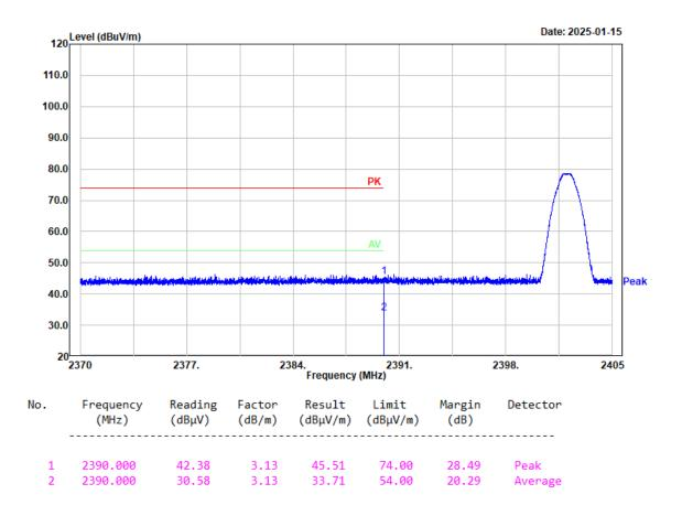
Project No.: 2403A43118E-RF Tester: coco Tian Condition: PK trace RBW:1MHz; VBW:3MHz; SWT:0.3sec Polarization: Vertical Note: 3EDR Low Channel 2402MHz Chain 1
