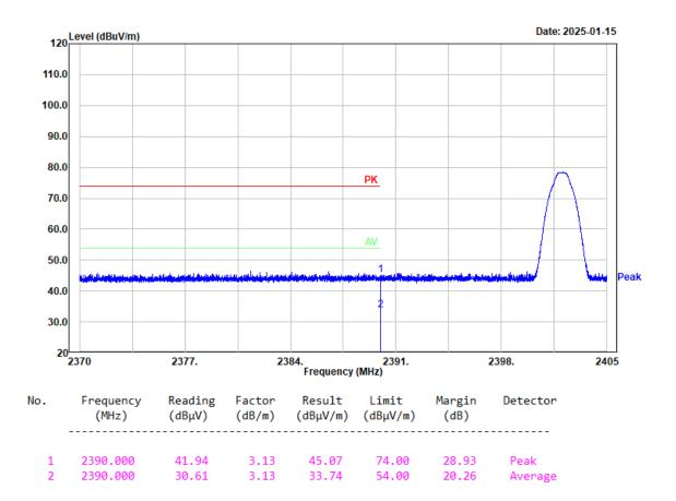
Project No.: 2403A43118E-RF Tester: coco Tian Condition: PK trace RBW:1MHz; VBW:3MHz; SWT:0.3sec Polarization: Vertical Note: 2EDR Low Channel 2402MHz Chain 1
