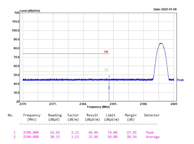
Project No.: 2403A43118E-RF Tester: coco Tian Condition: PK trace RBW:1MHz; VBW:3MHz; SWT:0.3sec Polarization: Horizontal Note: 3EDR High Channel 2480MHz Chain 0
