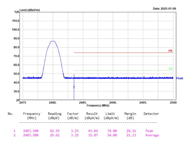
Project No.: 2403A43118E-RF Tester: coco Tian Condition: PK trace RBW:1MHz; VBW:3MHz; SWT:0.3sec Polarization: Horizontal Note: BDR Low Channel 2402MHz Chain 1
