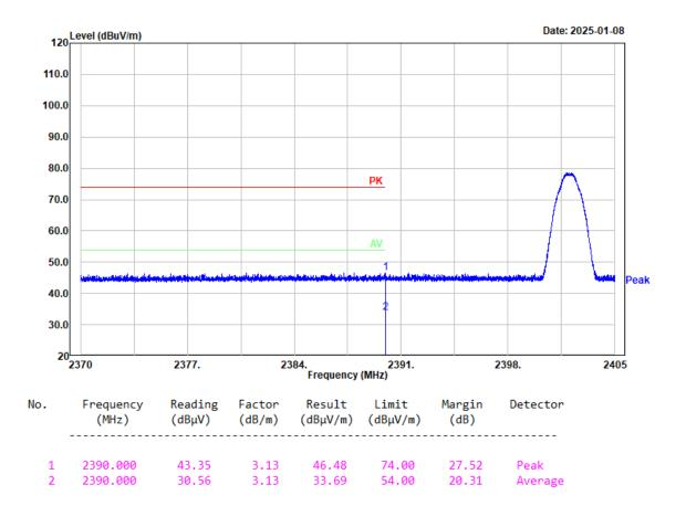
Project No.: 2403A43118E-RF Tester: coco Tian Condition: PK trace RBW:1MHz; VBW:3MHz; SWT:0.3sec Polarization: Vertical Note: 2EDR Low Channel 2402MHz Chain 0
