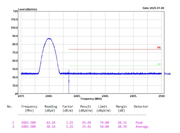
Project No.: 2403A43118E-RF Tester: coco Tian Condition: PK trace RBW:1MHz; VBW:3MHz; SWT:0.3sec Polarization: Horizontal Note: 2EDR Low Channel 2402MHz Chain 0
