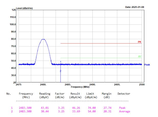
Project No.: 2403A43118E-RF Tester: coco Tian Condition: PK trace RBW:1MHz; VBW:3MHz; SWT:0.3sec Polarization: Vertical Note: 3EDR High Channel 2480MHz Chain 0
