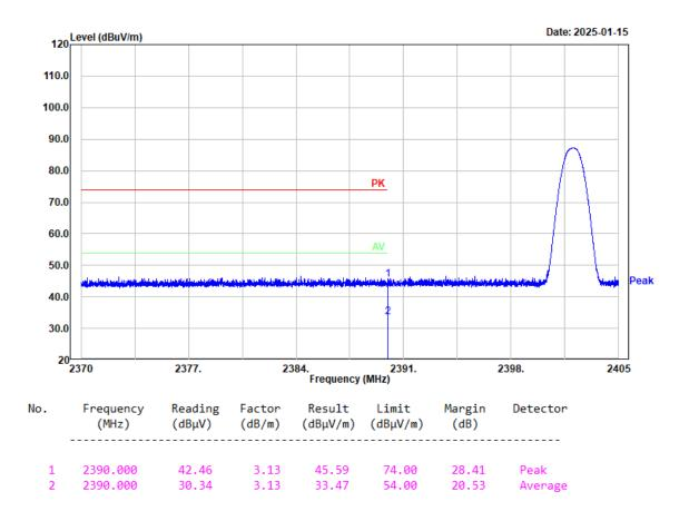
Project No.: 2403A43118E-RF Tester: coco Tian Condition: PK trace RBW:1MHz; VBW:3MHz; SWT:0.3sec Polarization: Horizontal Note: BDR High Channel 2480MHz Chain 1
