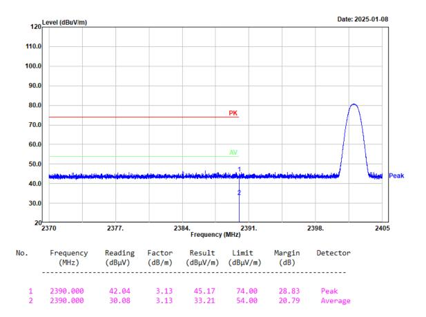
Project No.: 2403A43118E-RF Tester: coco Tian Condition: PK trace RBW:1MHz; VBW:3MHz; SWT:0.3sec Polarization: Vertical Note: BDR Low Channel 2402MHz Chain 0
