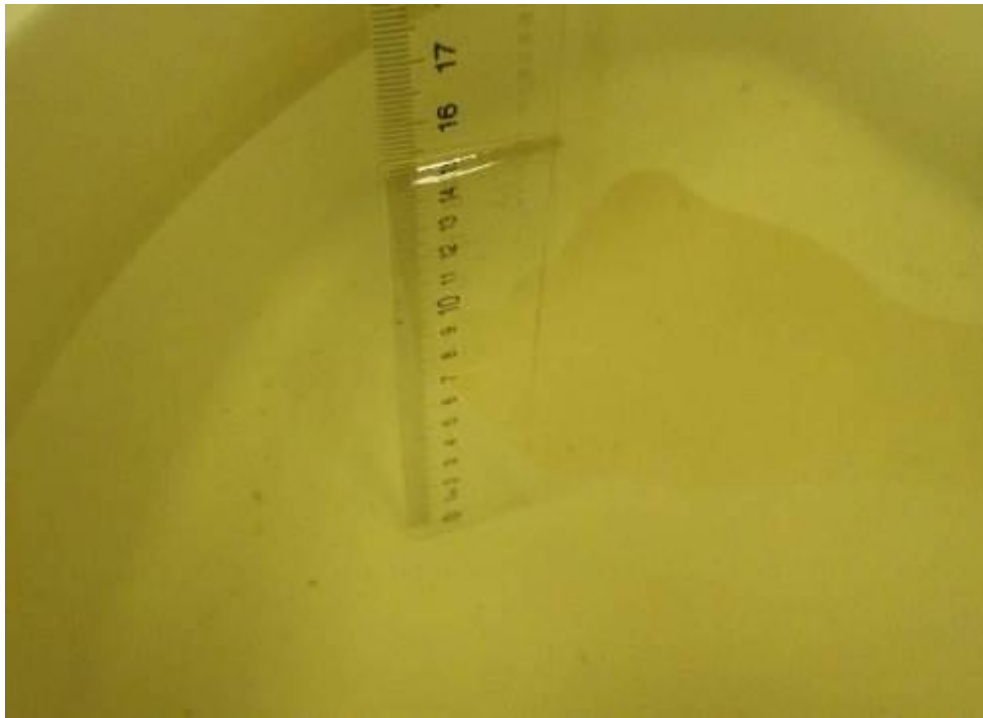
Picture 7-3: Liquid depth in the Flat Phantom (835 MHz Body)
