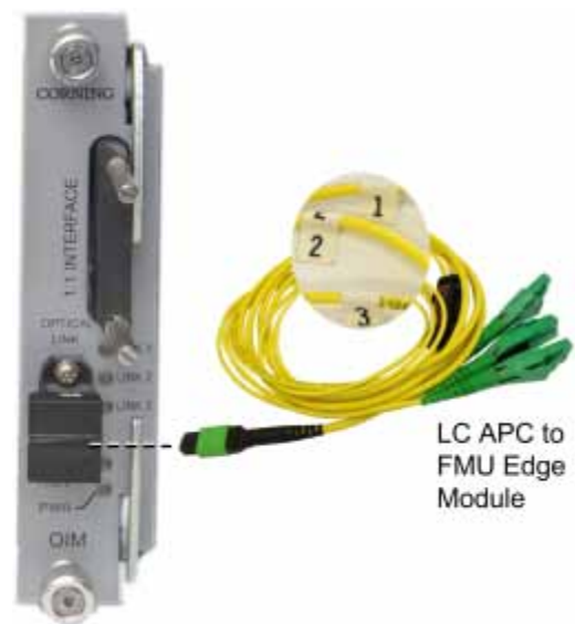
Figure 4-21. OIM Fiber Connections
