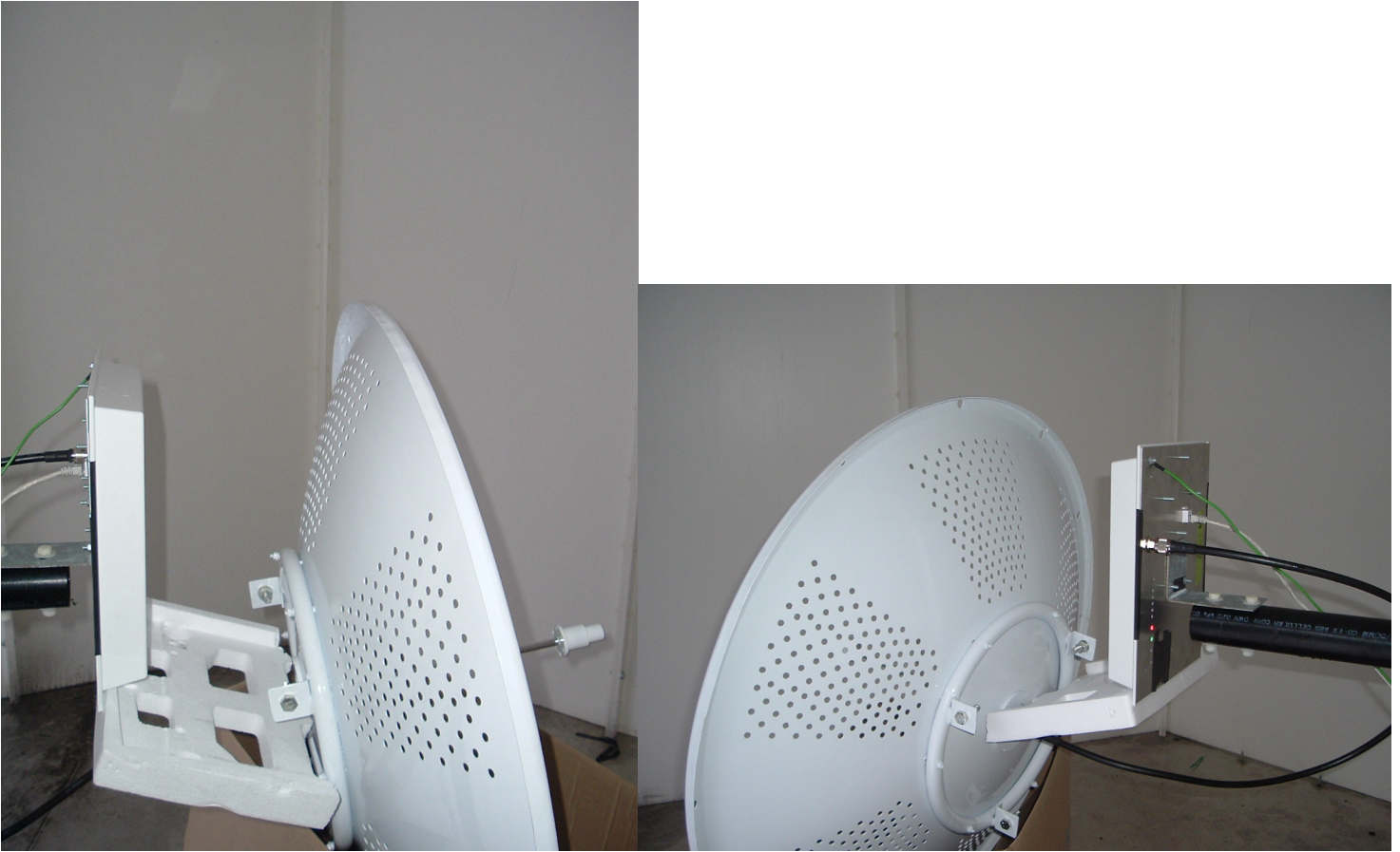
TR-AP5A-N with 32 dBi antenna.
