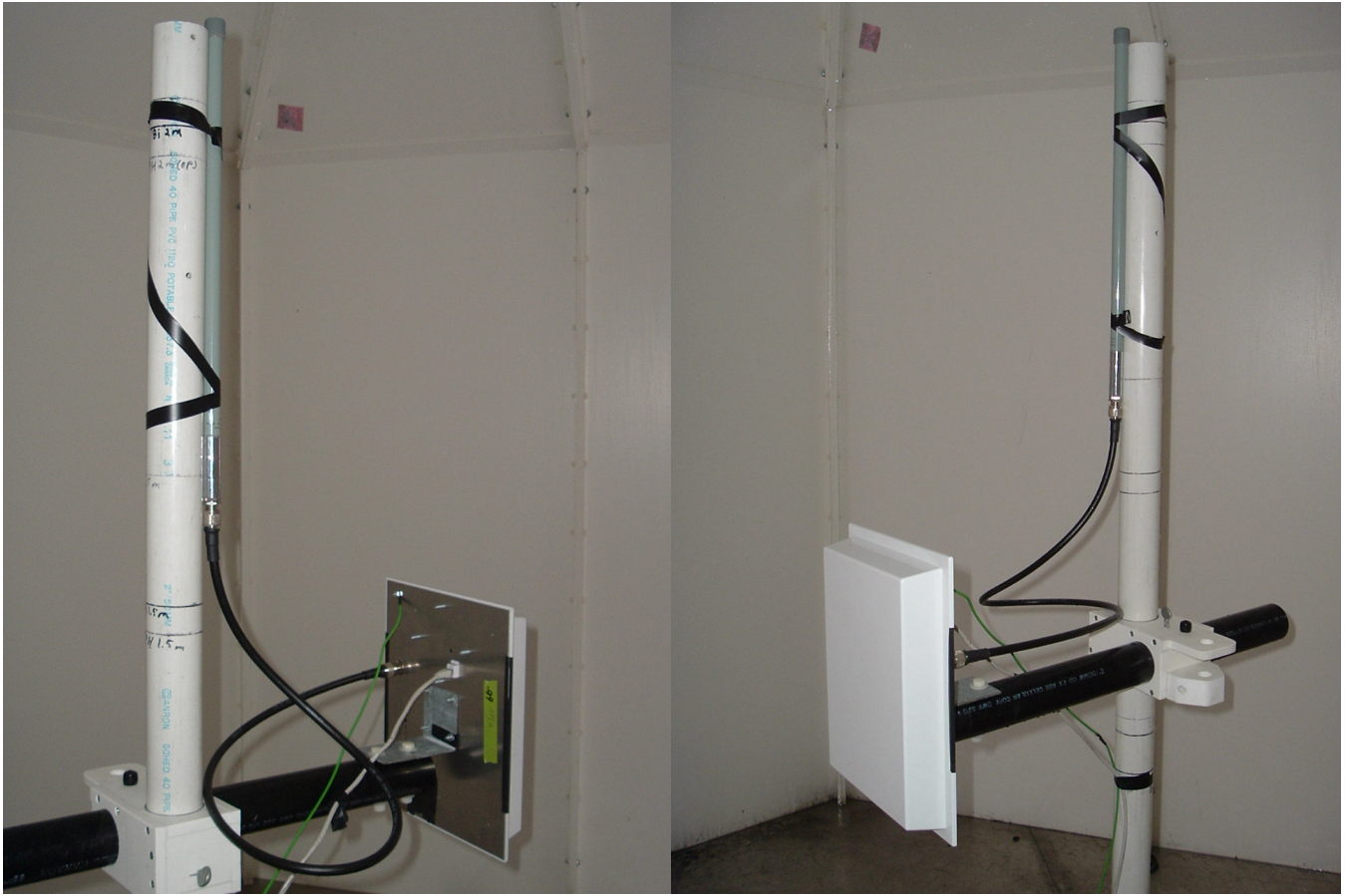
TR-AP5A-N with 12 dBi Antenna
