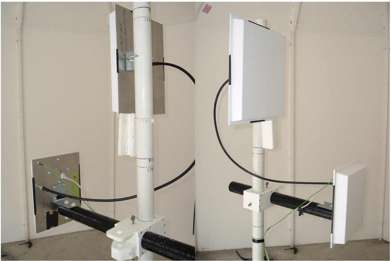
TR-AP5A-N with 24 dBi antenna
