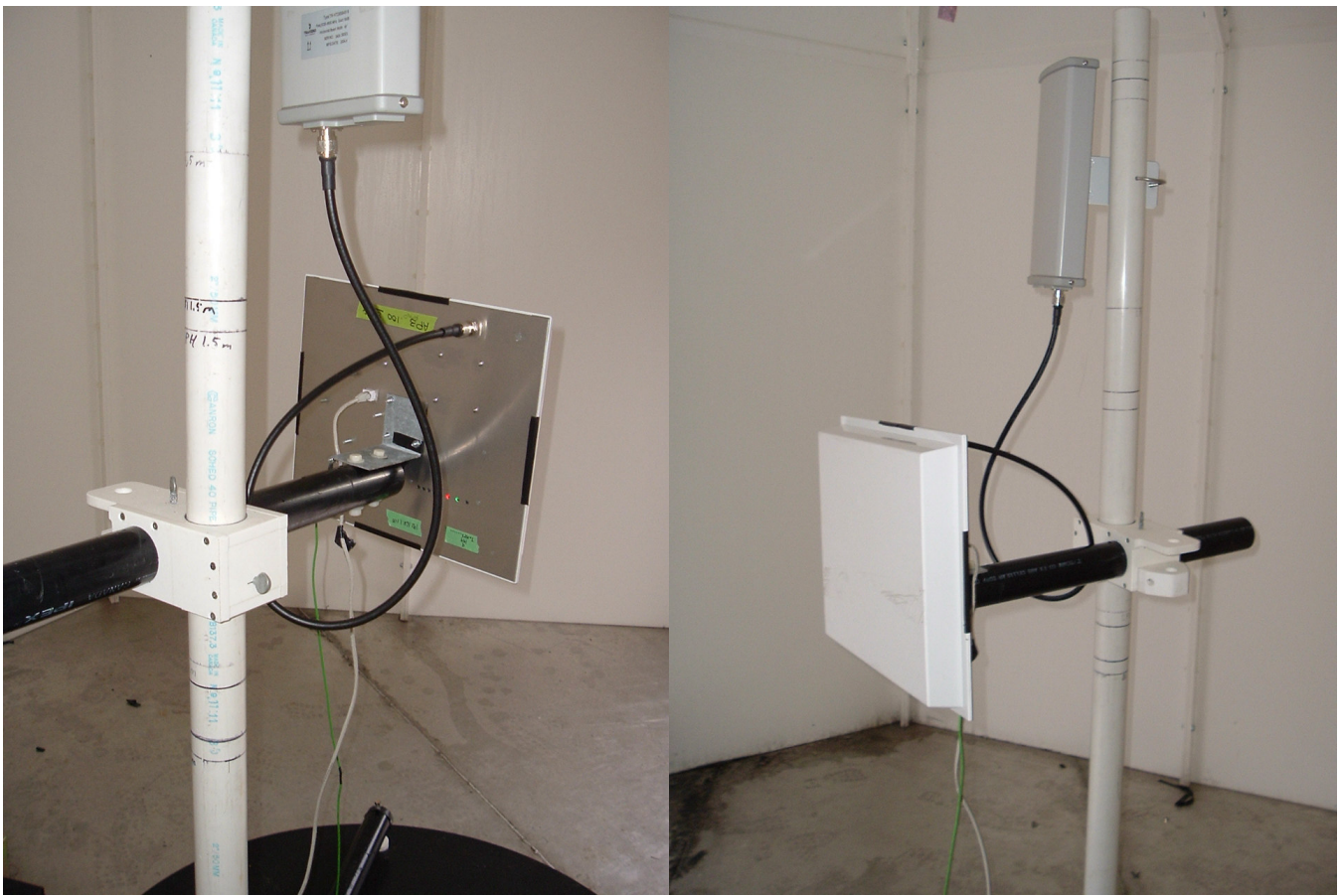
TR-AP5A-N with 19 dBi antenna
