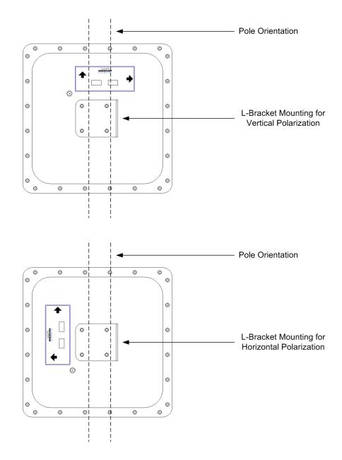
Once the L-bracket is in place, the unit can be mounted to the pole. The pole catch, V-bolt and L-bracket are oriented as shown in Diagrams 2.2B and 2.2C.
