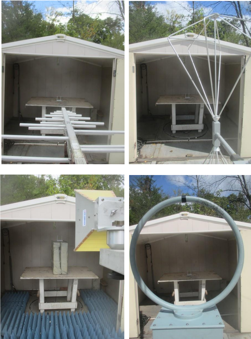
Figure 3.1 Radiated Test Setup
