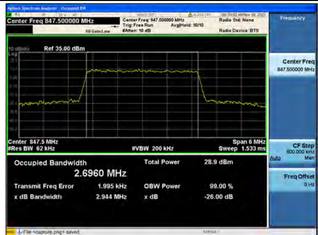
Band26Part22 / 3MHz / 64QAM/ High CH
