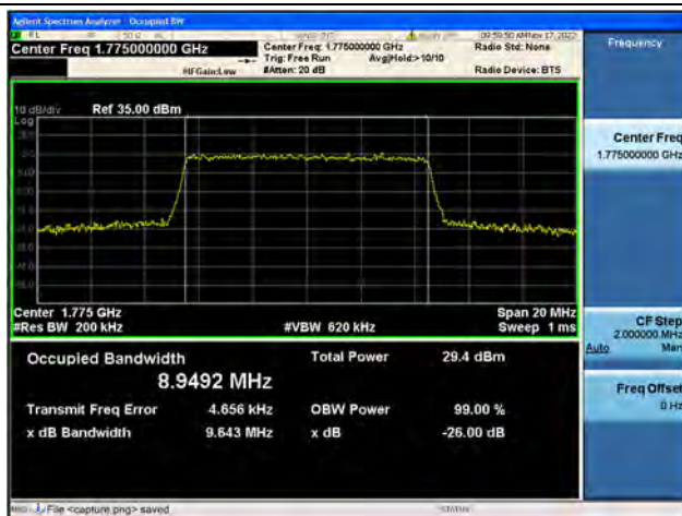
Band66 / 10MHz / 16QAM/ High CH
