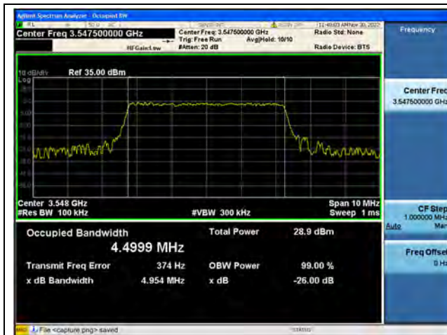
Band42 / 5MHz / QPSK/ High CH
