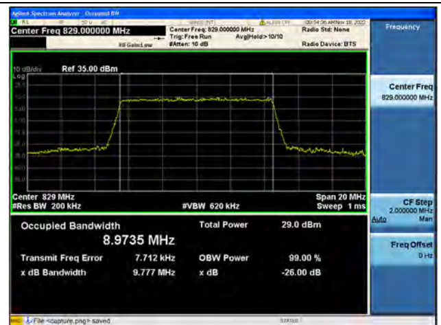
Band26Part22 / 10MHz / 64QAM/ Low CH
