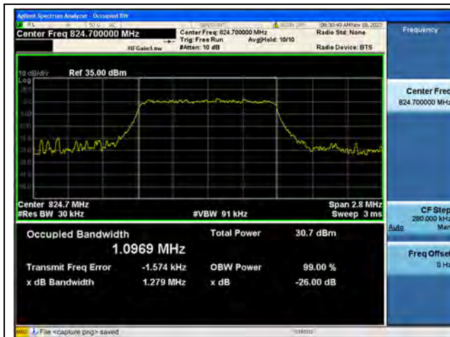
Band26Part22 / 1.4MHz / QPSK/ Low CH
