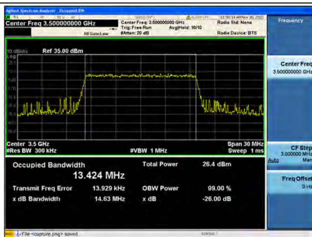
Band42 / 15MHz / 64QAM/ Mid CH
