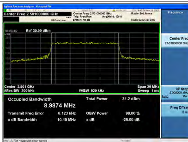
Band41 / 10MHz / 16QAM/ Low CH
