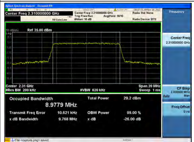
Band30 / 10MHz / 64QAM/ High CH
