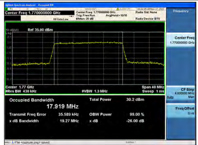
Band66 / 20MHz / QPSK/ High CH
