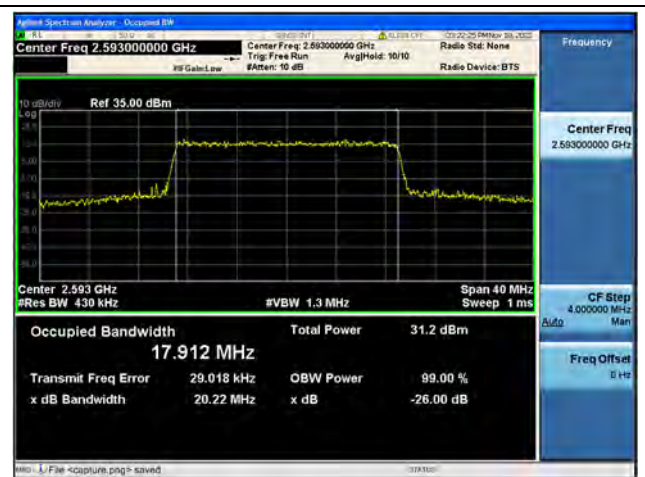
Band41 / 20MHz / 16QAM/ Mid CH
