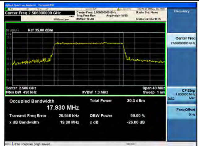
Band41 / 20MHz / 64QAM/ Low CH
