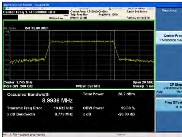
Band66 / 10MHz / 64QAM/ Mid CH
