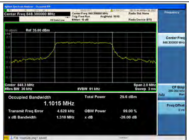
Band26Part22 / 1.4MHz / 16QAM / High CH
