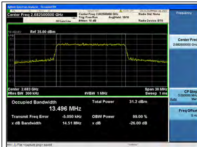
Band41 / 15MHz / QPSK/ High CH
