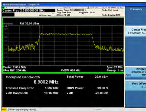
Band38 / 10MHz / 16QAM/ High CH
