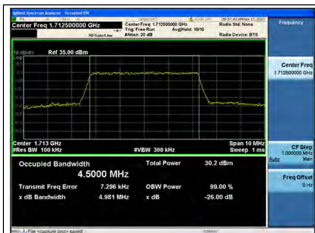
Band66 / 5MHz / QPSK/ Low CH
