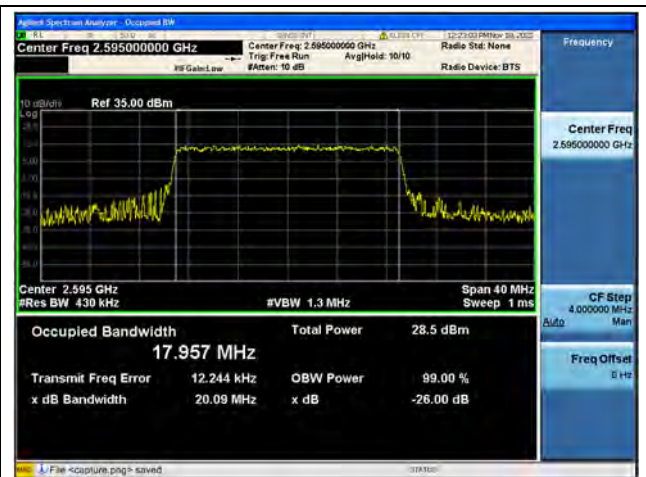
Band38 / 20MHz / 16QAM/ Mid CH
