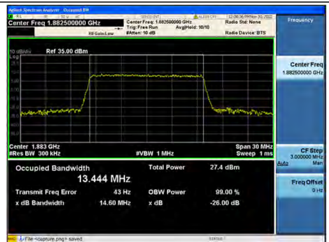
Band25 / 15MHz / 64QAM/ Mid CH
