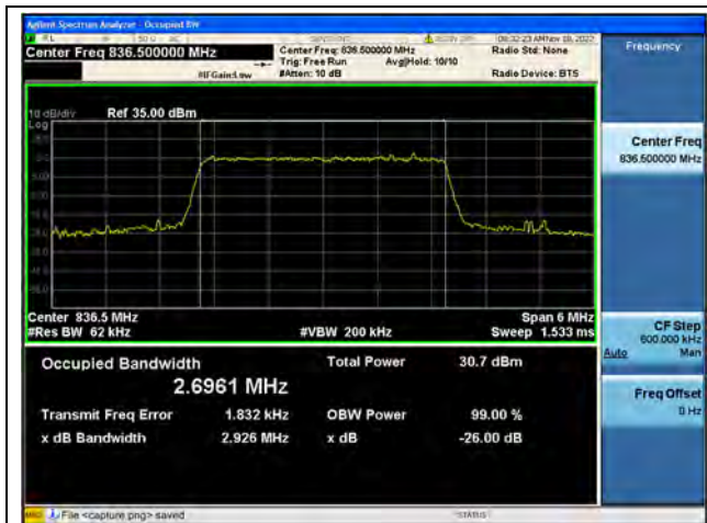
Band26Part22 / 3MHz / QPSK/ Mid CH
