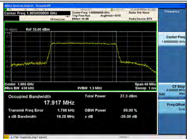
Band25 / 20MHz / 64QAM/ High CH
