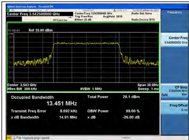
Band42 / 15MHz / QPSK/ High CH
