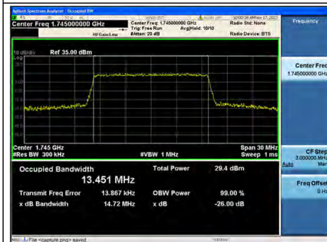
Band66 / 15MHz / 16QAM/ Mid CH
