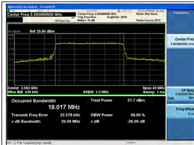
Band41 / 20MHz / QPSK/ Mid CH
