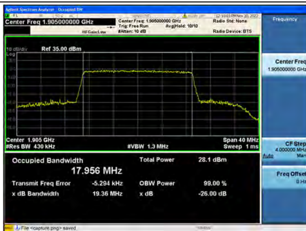
Band25 / 20MHz / 16QAM/ High CH
