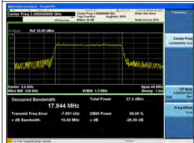
Band42 / 20MHz / 64QAM/ Mid CH
