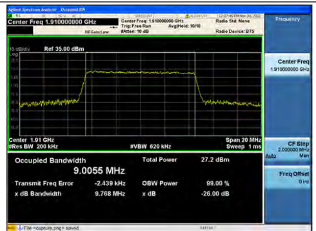
Band25 / 10MHz / 64QAM/ High CH
