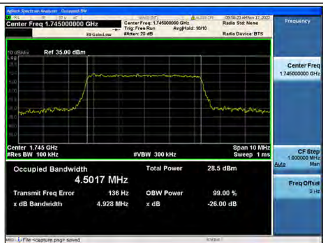
Band66 / 5MHz / 64QAM/ Mid CH
