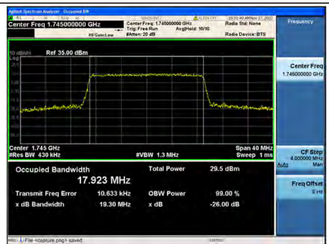
Band66 / 20MHz / 16QAM/ Mid CH
