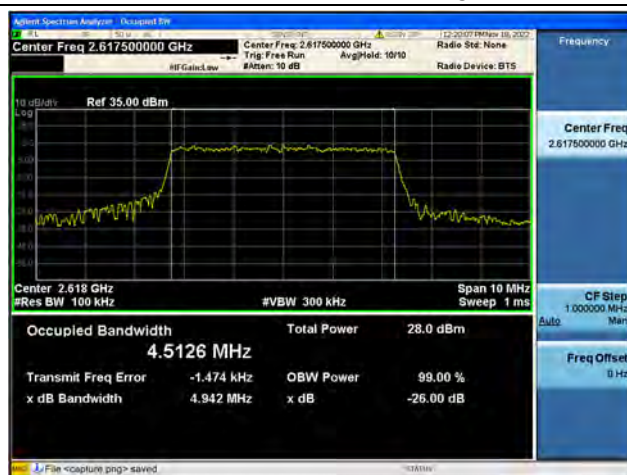
Band38 / 5MHz / 64QAM/ High CH
