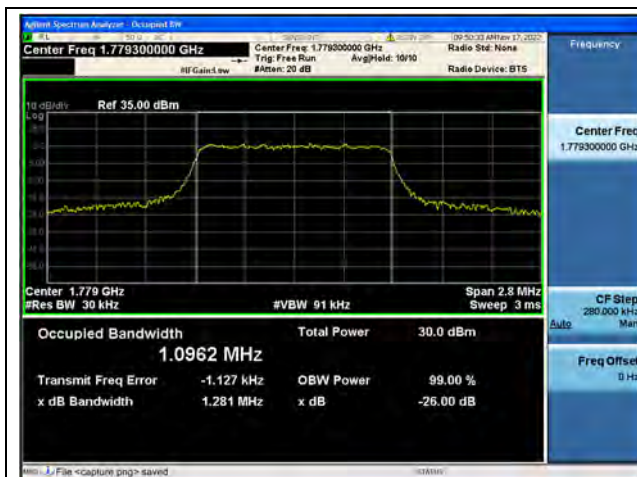
Band66 / 1.4MHz / QPSK/ High CH
