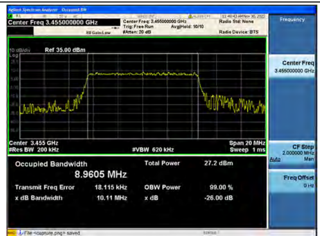
Band42 / 10MHz / 64QAM/ Low CH
