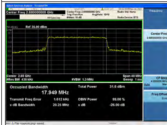
Band41 / 20MHz / 16QAM/ High CH
