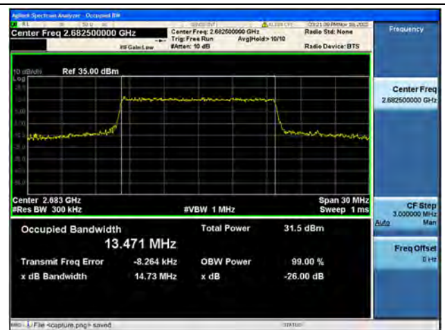
Band41 / 15MHz / 16QAM/ High CH
