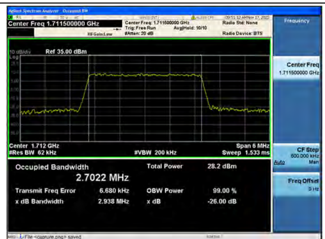
Band66 / 3MHz / 64QAM/ Low CH
