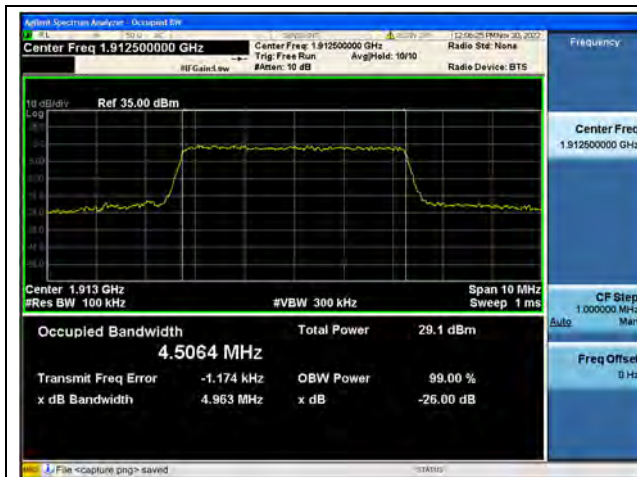
Band25 / 5MHz / QPSK/ High CH
