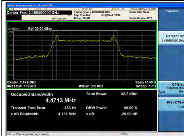
Band41 / 5MHz / 64QAM/ Low CH
