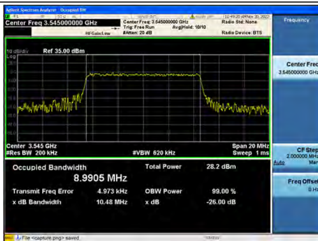
Band42 / 10MHz / 16QAM/ High CH
