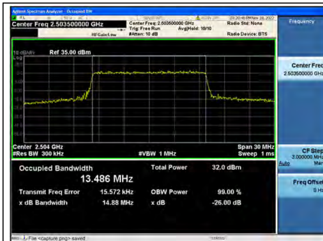
Band41 / 15MHz / QPSK/ Low CH
