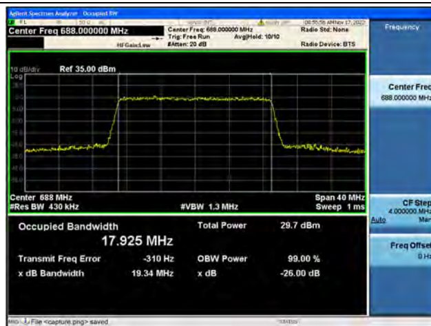
Band71 / 20MHz / 16QAM/ High CH
