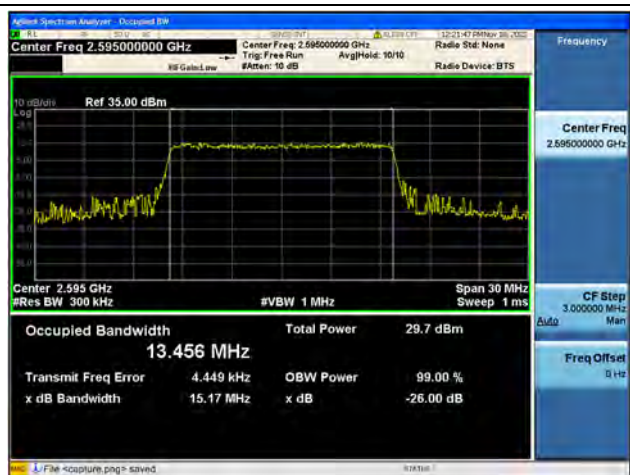
Band38 / 15MHz / QPSK/ Mid CH
