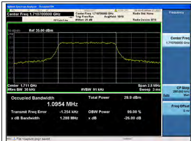
Band66 / 1.4MHz / QPSK/ Low CH
