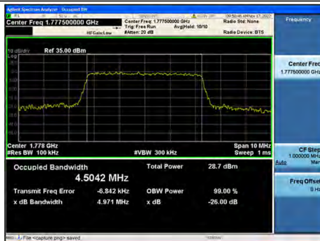
Band66 / 5MHz / 64QAM/ High CH
