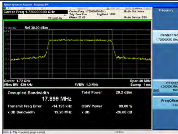
Band66 / 20MHz / 16QAM/ Low CH
