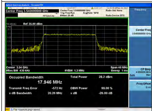
Band42 / 20MHz / 16QAM/ High CH
