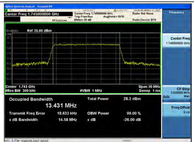
Band66 / 15MHz / 64QAM/ Mid CH
