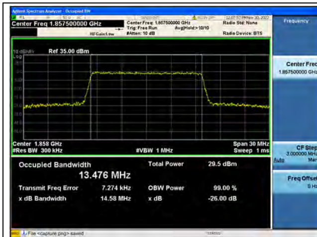
Band25 / 15MHz / QPSK/ Low CH
