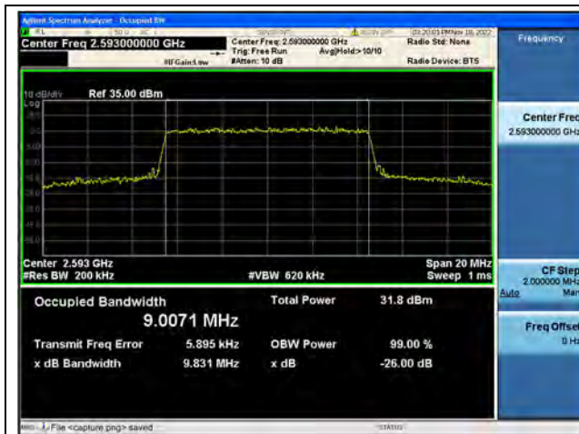
Band41 / 10MHz / QPSK/ Mid CH
