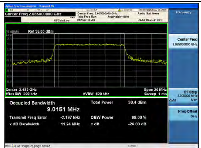
Band41 / 10MHz / 64QAM/ High CH
