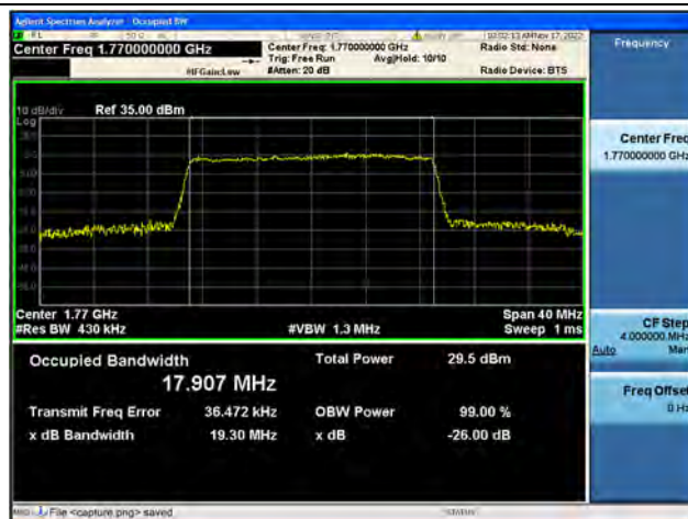
Band66 / 20MHz / 16QAM/ High CH
