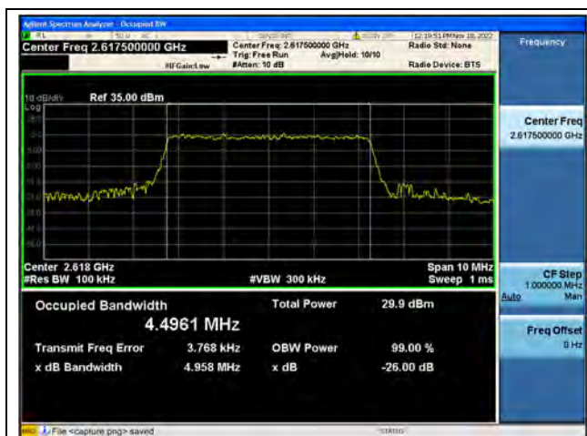
Band38 / 5MHz / QPSK/ High CH
