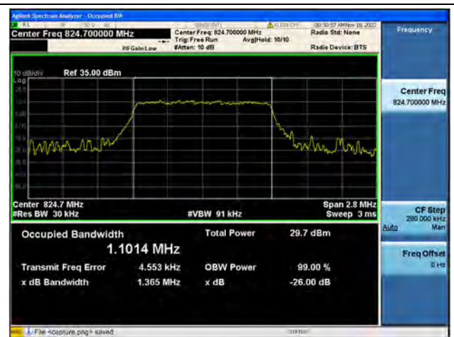
Band26Part22 / 1.4MHz / 16QAM/ Low CH
