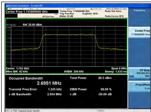
Band66 / 3MHz / QPSK/ Mid CH
