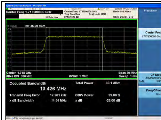
Band66 / 15MHz / QPSK/ Low CH
