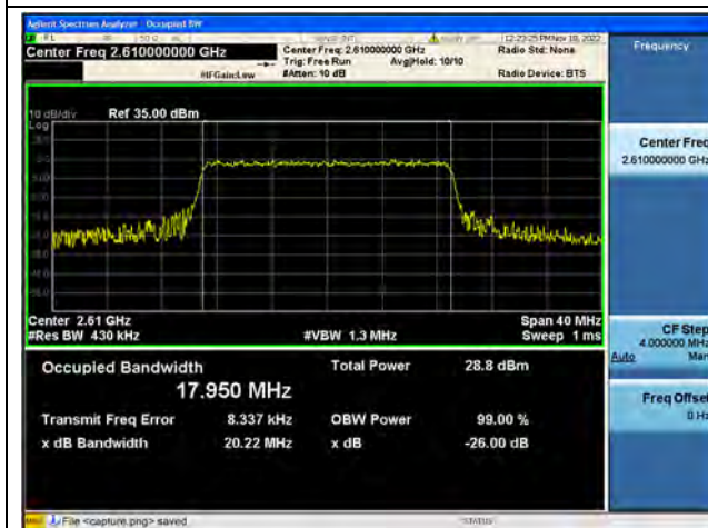
Band38 / 20MHz / 16QAM/ High CH
