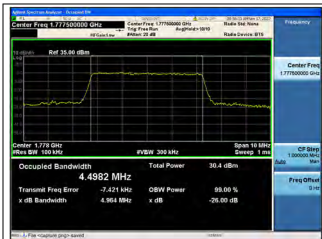
Band66 / 5MHz / QPSK/ High CH
