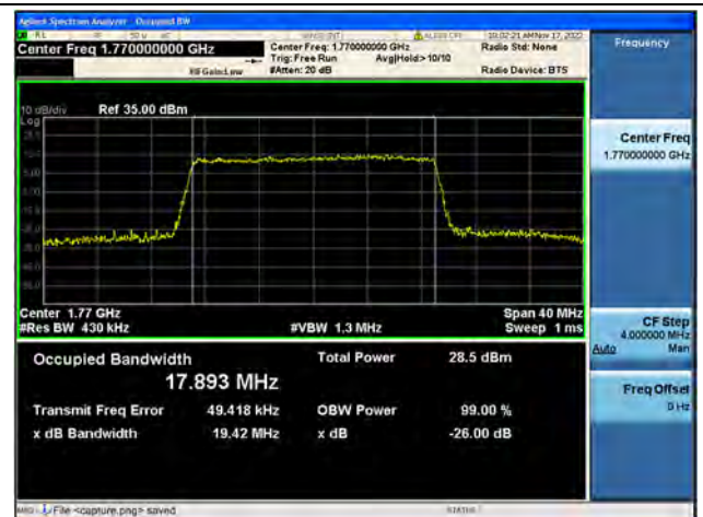
Band66 / 20MHz / 64QAM/ High CH
