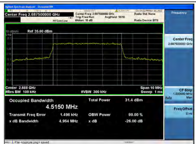
Band41 / 5MHz / 16QAM/ High CH
