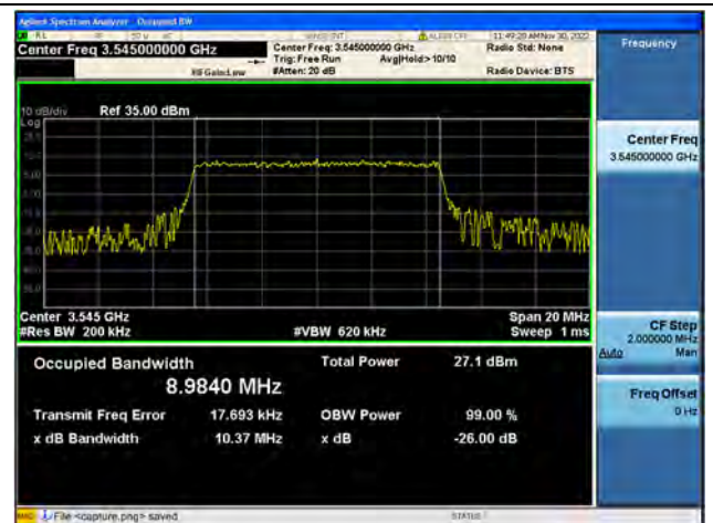
Band42 / 10MHz / 64QAM/ High CH
