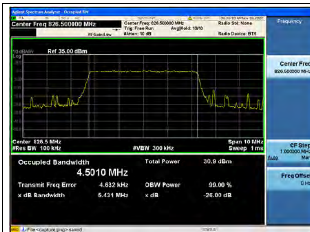
Band26Part22 / 5MHz / QPSK/ Low CH
