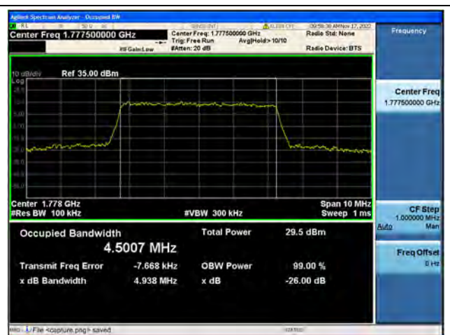
Band66 / 5MHz / 16QAM/ High CH
