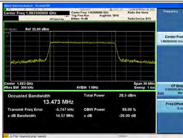
Band25 / 15MHz / 16QAM/ Mid CH
