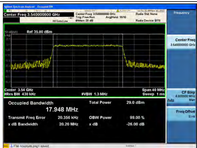
Band42 / 20MHz / QPSK/ High CH
