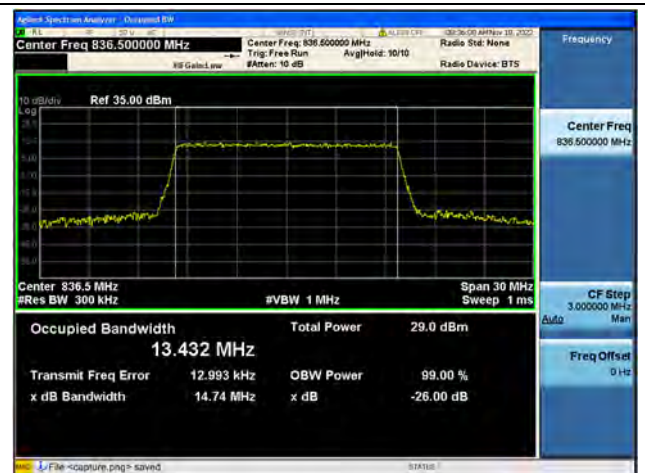
Band26Part22 / 15MHz / 64QAM/ Mid CH
