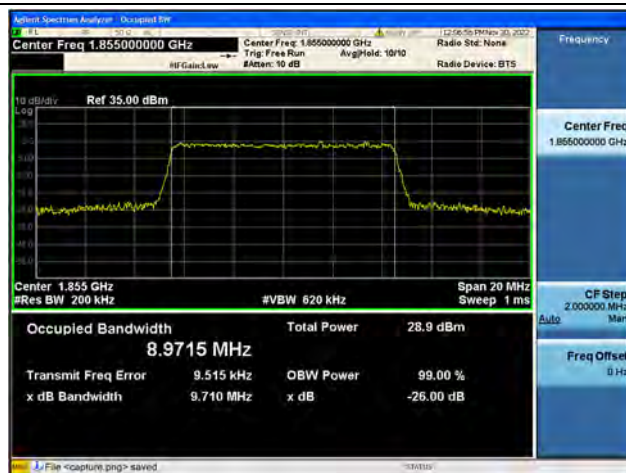
Band25 / 10MHz / 16QAM/ Low CH
