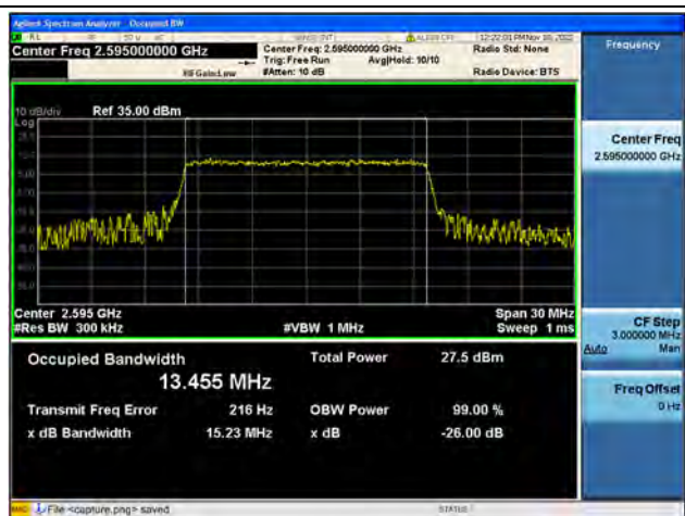
Band38 / 15MHz / 64QAM/ Mid CH
