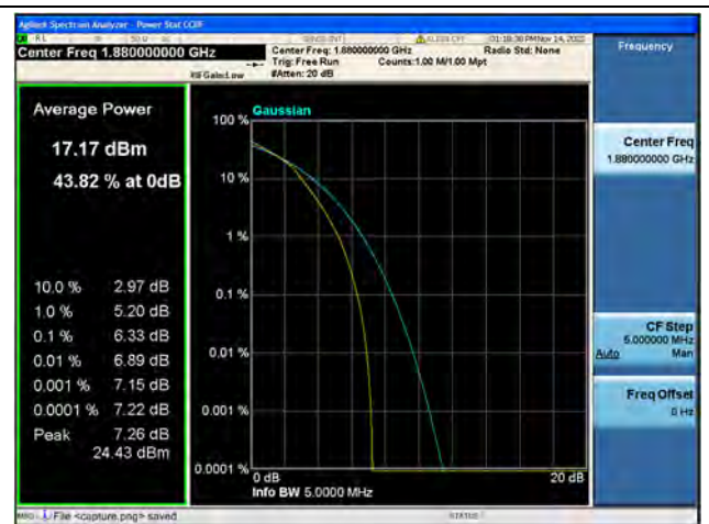
Band2 / 3MHz / Mid CH / 16QAM
