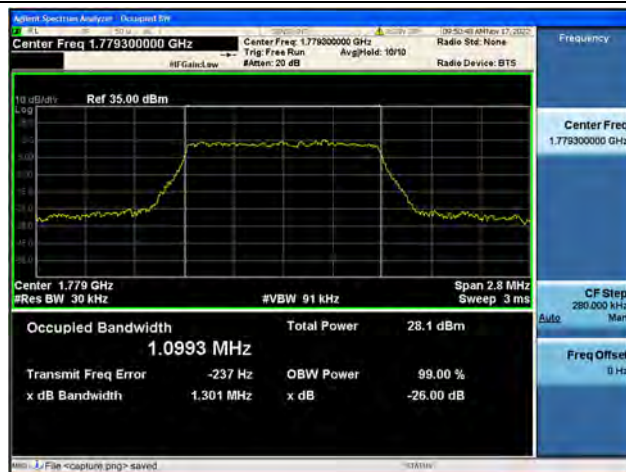
Band66 / 1.4MHz / 64QAM/ High CH
