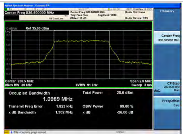
Band26Part22 / 1.4MHz / 64QAM/ Mid CH
