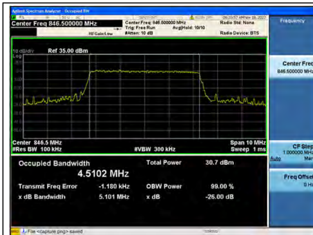
Band26Part22 / 5MHz / QPSK/ High CH
