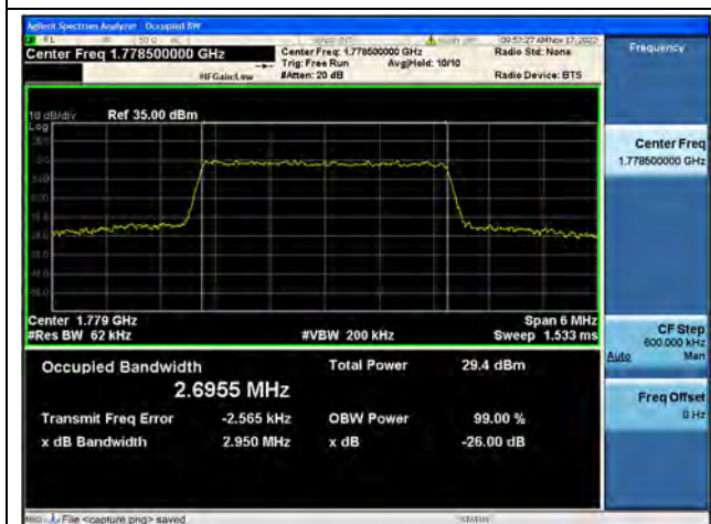
Band66 / 3MHz / 16QAM/ High CH
