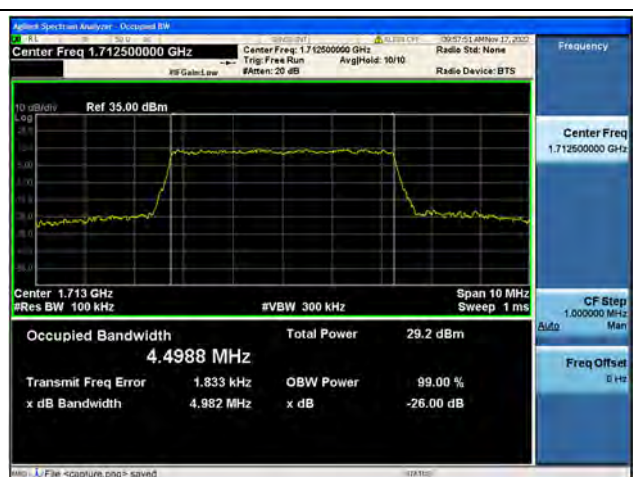
Band66 / 5MHz / 16QAM/ Low CH
