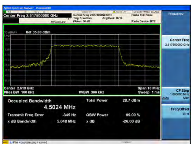
Band38 / 5MHz / 16QAM/ High CH
