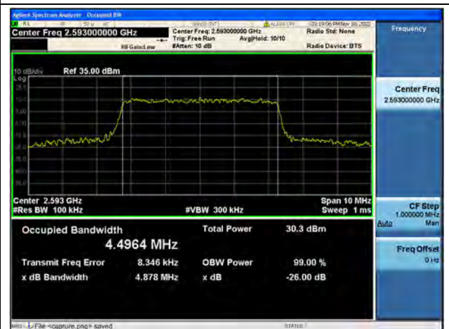
Band41 / 5MHz / 64QAM/ Mid CH
