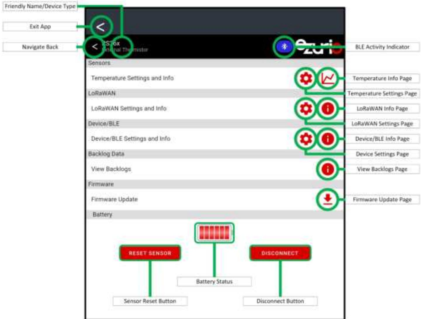
**Figure 10: RS26x Sensor Applet Device Home page**
