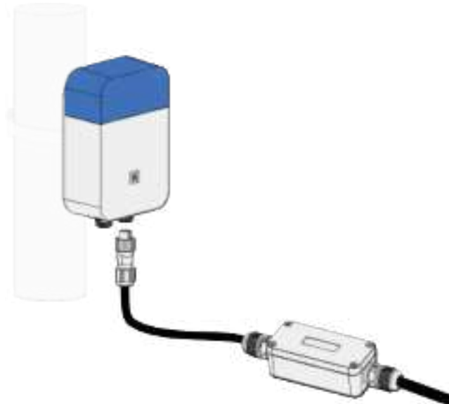
Figure 22: Connection the Probe IO to the Hub
