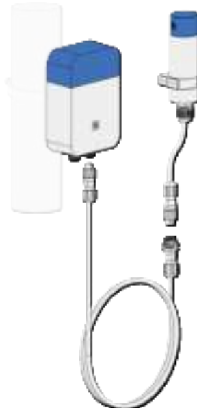
Figure 15: Connection via an extender
