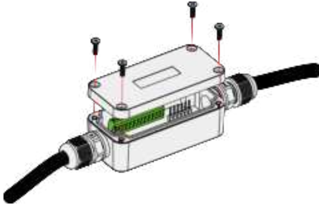
Figure 21: Closing the Probe IO
