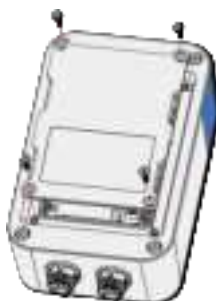
Figure 1: Removing the back cover
