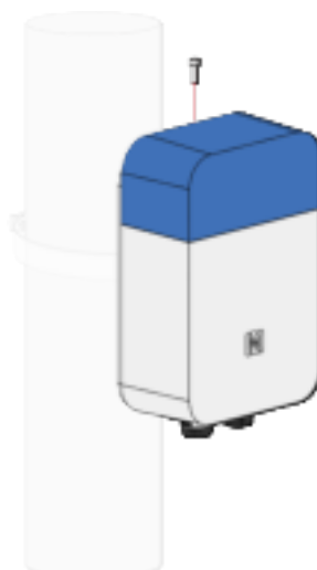
Figure 9: Adding a security screw
