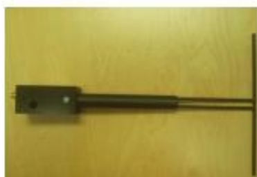
Figure 1 – MVG COMOSAR Validation Dipole
