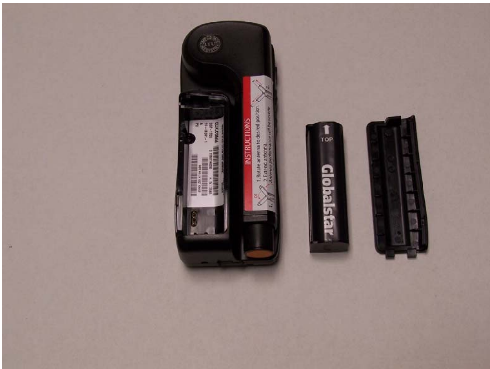
Figure 9 UT External- Battery Compartment Open
