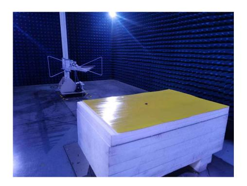
Photo of Radiated Emission Measurement Above 1GHz
