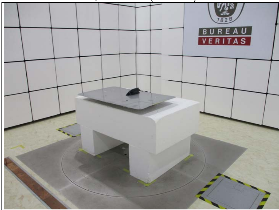
Radiated Emission Test (Below 1GHz) EUT + Antenna 2 (2nd Source)
