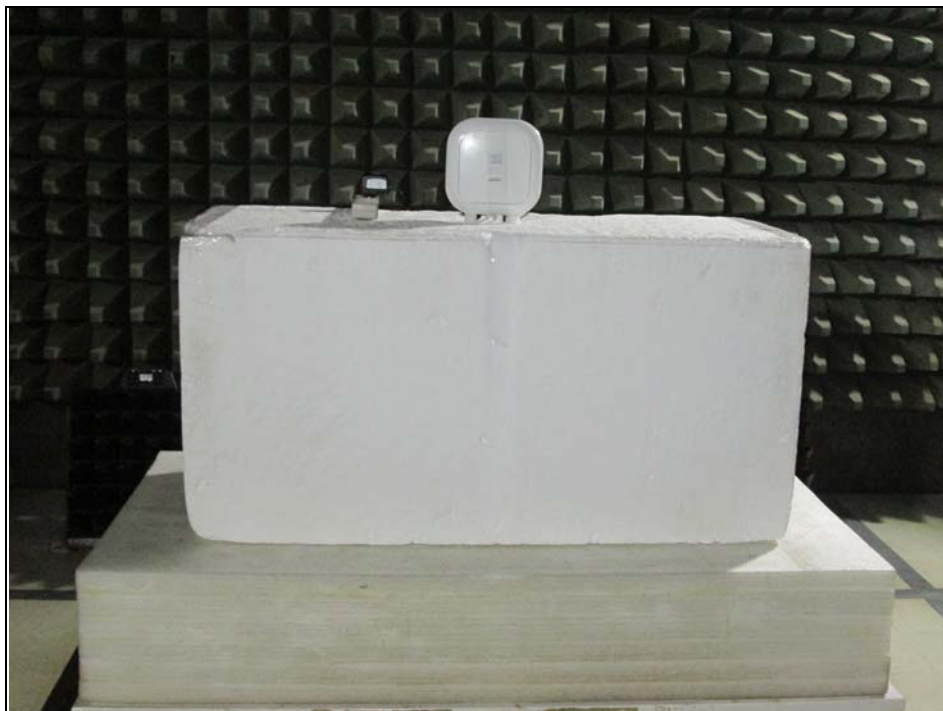
Radiated Emission Test (Above 1GHz)
