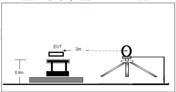
(B) Radiated Emission Test-Up Frequency 30MHz~1GHz
