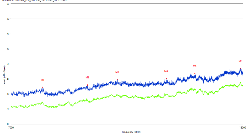
REmission Test case_FCC_Part 15C_FCC 15.247.7GHz-18GHz
