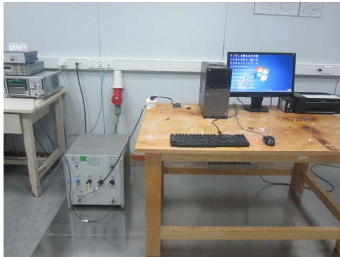
Radiated Emission (30MHz-1GHz) Connect to PC
