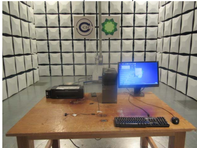
Radiated Emission (above 1GHz) Connect to PC
