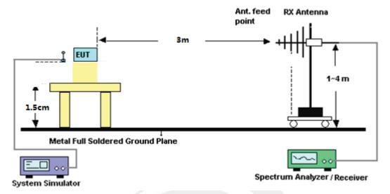
For radiated test from above 1GHz
