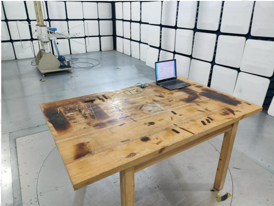
Photo of Radiation Emission Test
