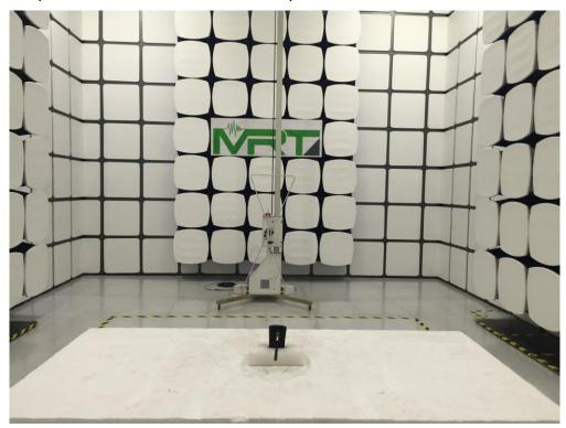
Description: Radiated Emission Test Setup for 1GHz ~ 10GHz
