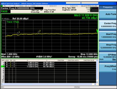
Transmitter Radiated Emission (2.4GHz Wi-Fi All modes)
