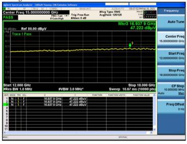
Transmitter Radiated Emission (2.4GHz Auxiliary Radio All modes)
