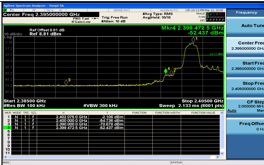
Band-edge for RF Conducted Emissions_3DH5_2402_Hopping On
