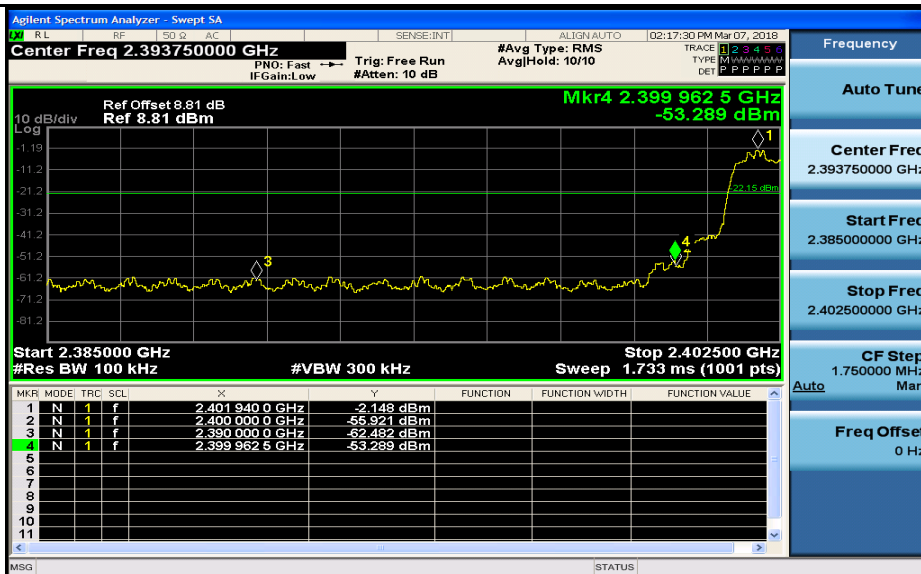
Band-edge for RF Conducted Emissions_2DH5_2480_Hopping Off
