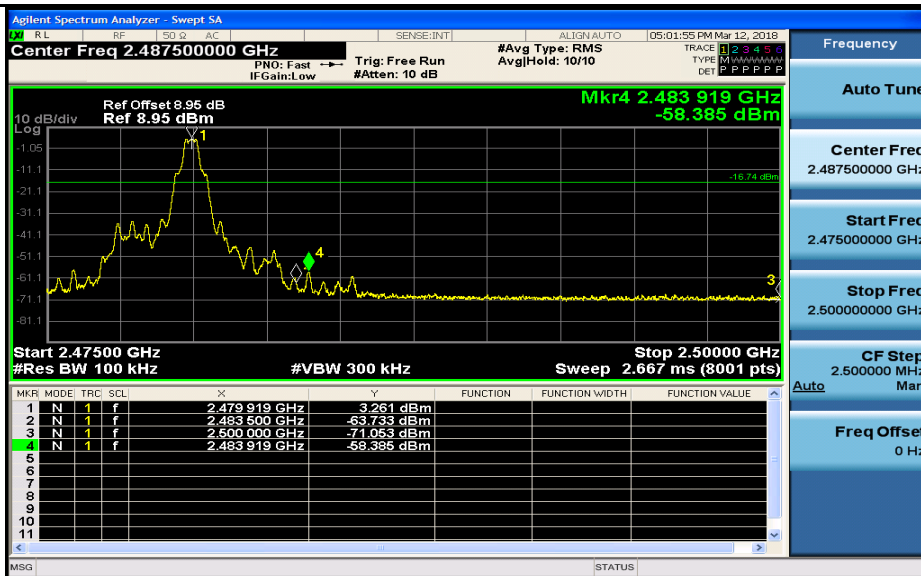
Band-edge for RF Conducted Emissions_DH5_2480_Hopping On
