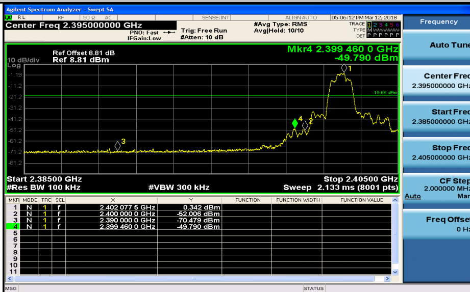
Band-edge for RF Conducted Emissions_2DH5_2402_Hopping On
