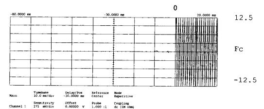
Trigger mode : Edge On Positive Edge Of Chan2 Trigger Level Chan2 - 600,000 mV (noise reject ON) Holdoff - 40,000 ns
