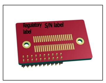
An auxiliary label will be provided for systems using the module where the original label not will be visible when the module is installed.
