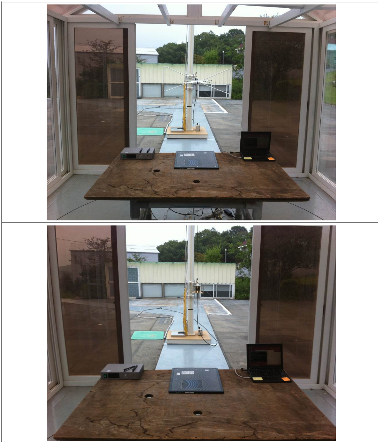
Figure.1. Radiated Emission Test Setup
