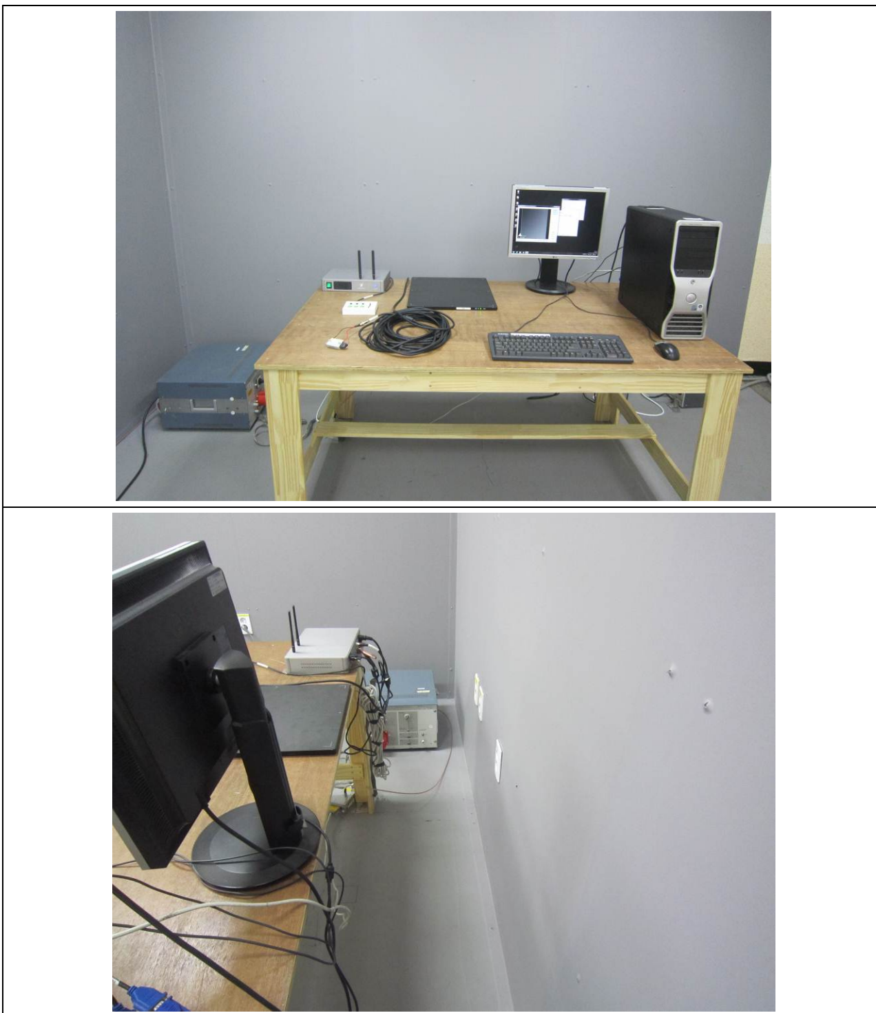
Figure.2. Test Setup for Conducted Emissions
