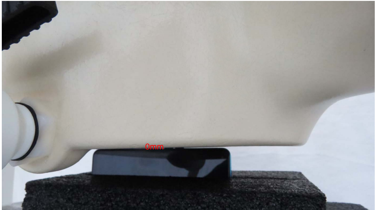
Picture 15: Right Side, the distance from handset to the bottom of the Phantom is 0mm
