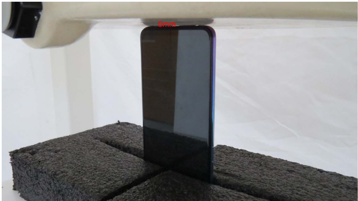
Picture 20: Bottom Edge, the distance from handset to the bottom of the Phantom is 0mm
