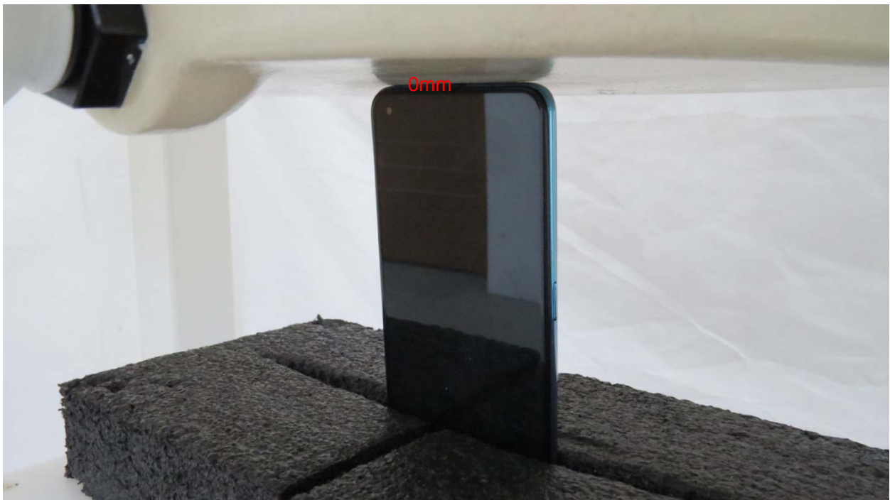
Picture 18: Top Side, the distance from handset to the bottom of the Phantom is 0mm
