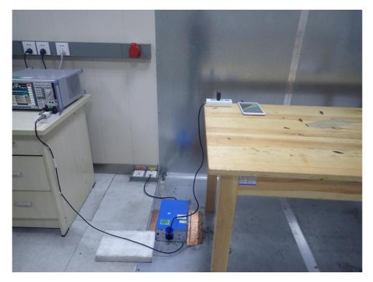
RADIATED EMISSION TEST SETUP
