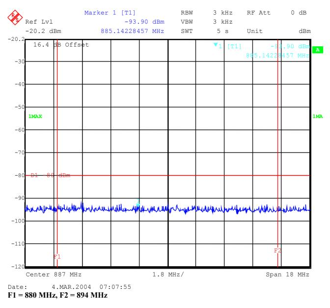
LIMITS §22.917(f) The mean power of any emissions appearing in the base station frequency range from cellular mobile transmitters operated must be attenuated to a level not to exceed –80dBm at the transmitter antenna connector
