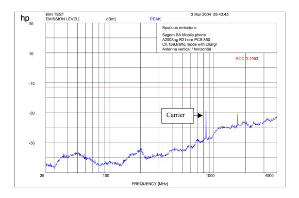
f < 1 GHz: RBW/VBW: 100 kHz  $f \ge 1 \text{ GHz}$ : RBW/VBW 1 MHz Carrier suppressed with a rejection filter
