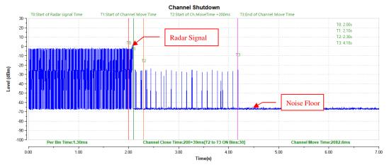
NOTE: Zoom in of the first 7000ms after radar signal applied.
