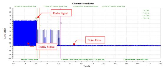
NOTE: T1 denotes the start of Channel Move Time upon the end of the last Radar burst. T2 denotes the data transmission time of 200ms from T1. T3 denotes the end of Channel Move Time.
