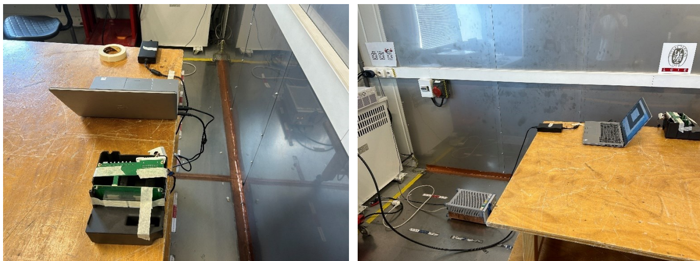
Photo of AC Power Line Conducted Emissions
