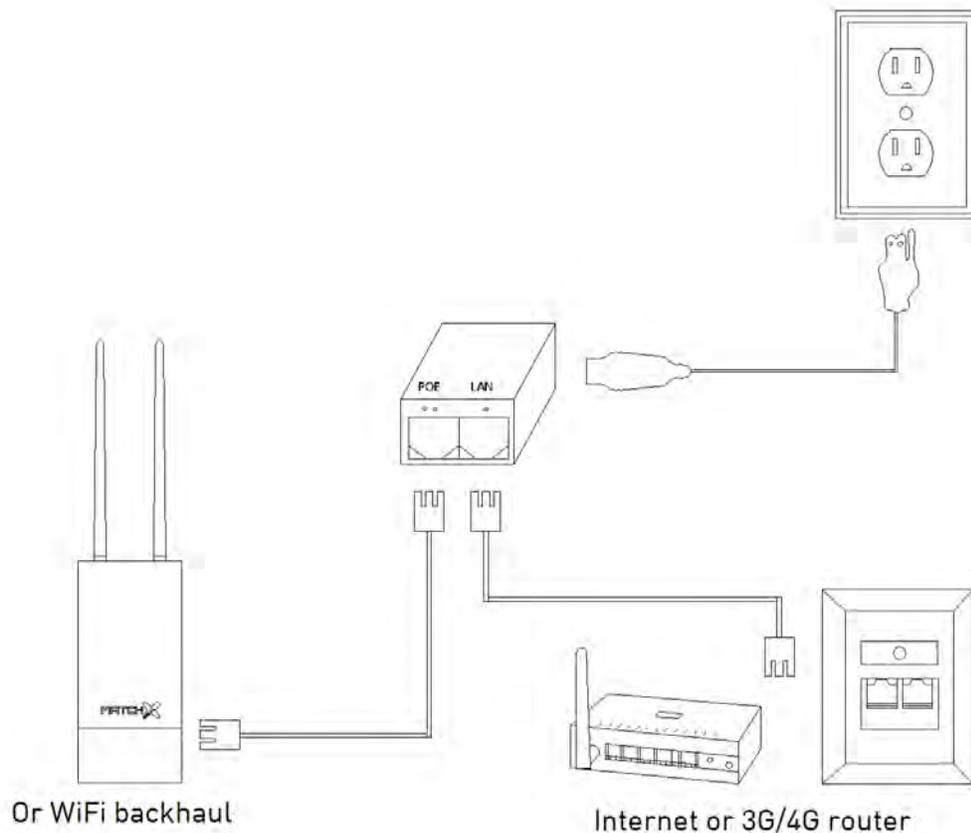
Firstly connect to power cords from your wall sockets or panel sockets to POE, then connect the RJ45 cable from your Internet modem/switch/wall port, or any 3G/4G router to the POE's port labeled with "LAN". Next, grab a RJ45 cable and connect from the POE's port labeled with "POE" to Box.
