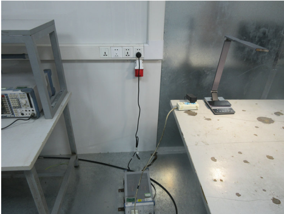
Photo of Conducted Emission Measurement
