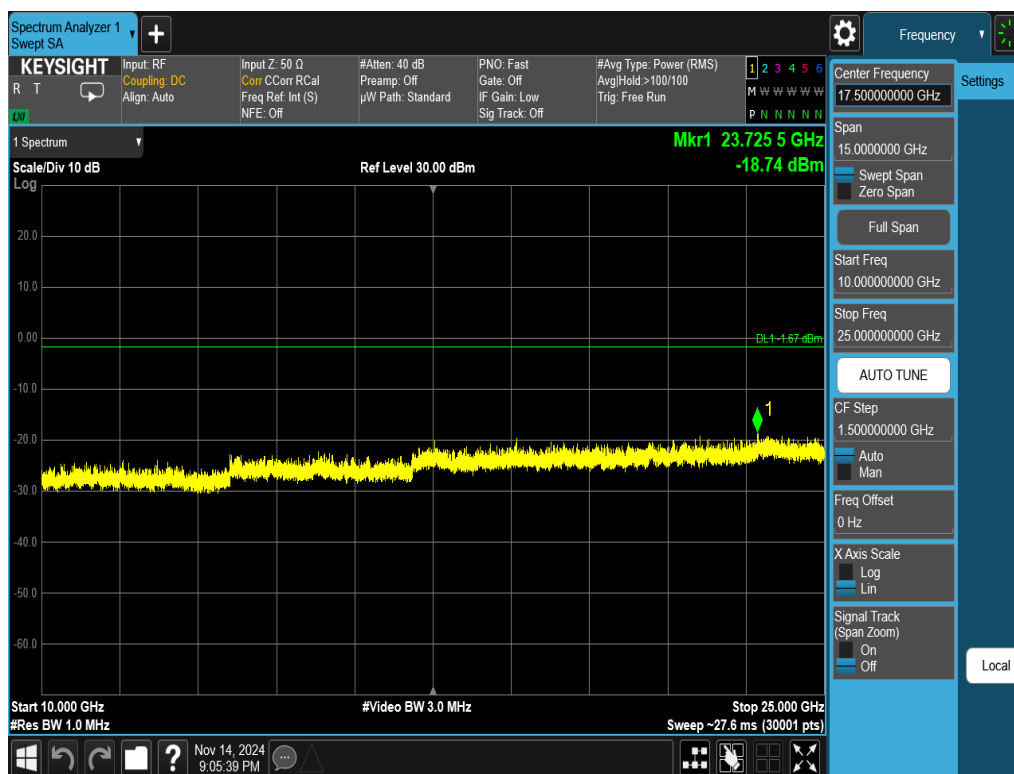
Plot 7-48. Conducted Spurious Plot Antenna WF8 (802.11ax OFDMA – RU26 – Ch. 11)
