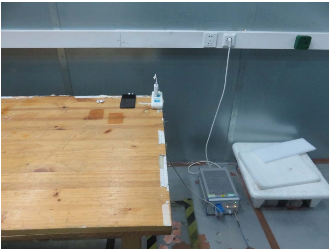
Picture 2 Conducted Emission Test Setup
