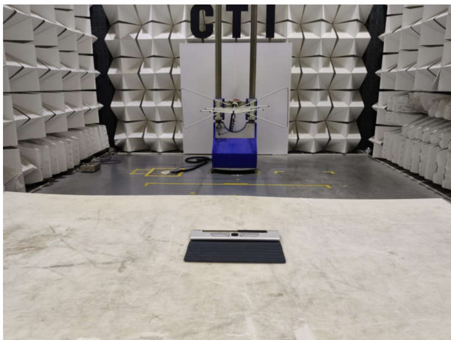
Radiated spurious emission Test Setup-2(Below 1GHz)
