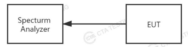
The EUT is connected to the Spectrum Analyzer; the RF load attached to the EUT antenna terminal is 500hm; the path loss as the factor is calibrated to correct the reading. Make the measurement with the spectrum analyzer's resolution bandwidth (RBW) = 100 kHz. In
