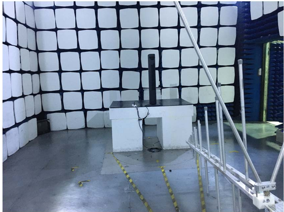
Radiation Emission Test Setup (30MHz to 1GHz)
