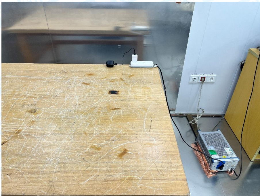
Photo of Setup for Conducted Emission
