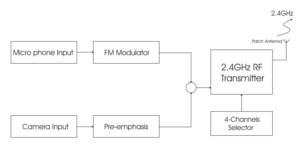
Block Diagram for Indoor/Outdoor Color Video Camera With Built-in 2.4 GHz Transmitter(XX10A)
