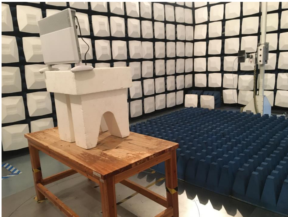
Test Setup For Radiated Emission (Above 1GHz)
