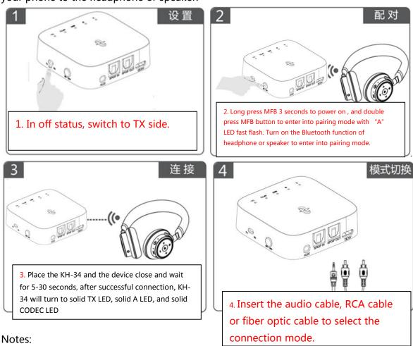
CODEC indicator flash in different way depend on different CODEC (of connected device) after connected, refer to point 6 LED indicator.
