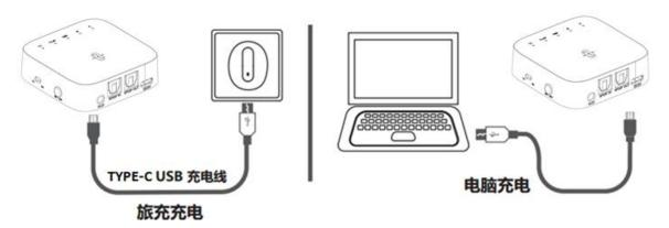
Charging with Type-C USB cable / Charging with PC
