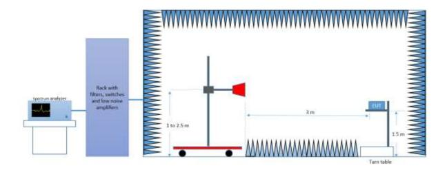
Radiated Setup 18 GHz - 40 GHz
