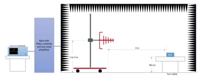
Radiated Setup 1 GHz - 18 GHz
