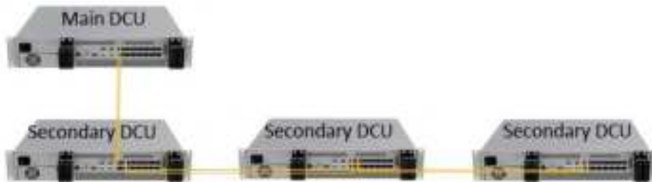
Figure 11. DCU Daisy Connection
