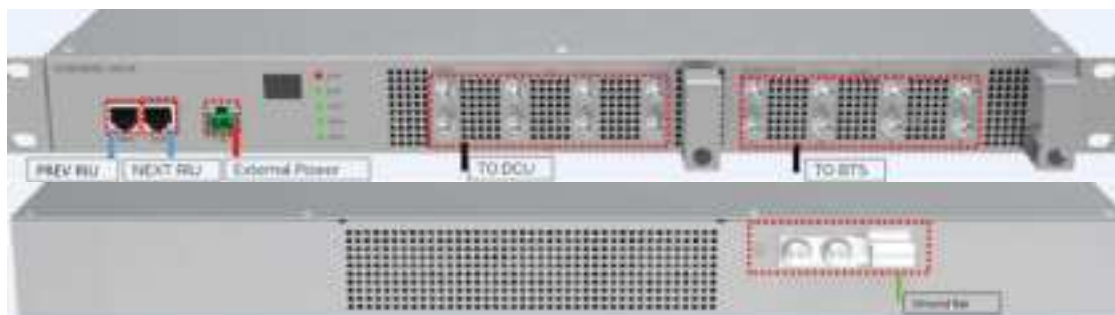
Figure 27. RIU Cable Connection
