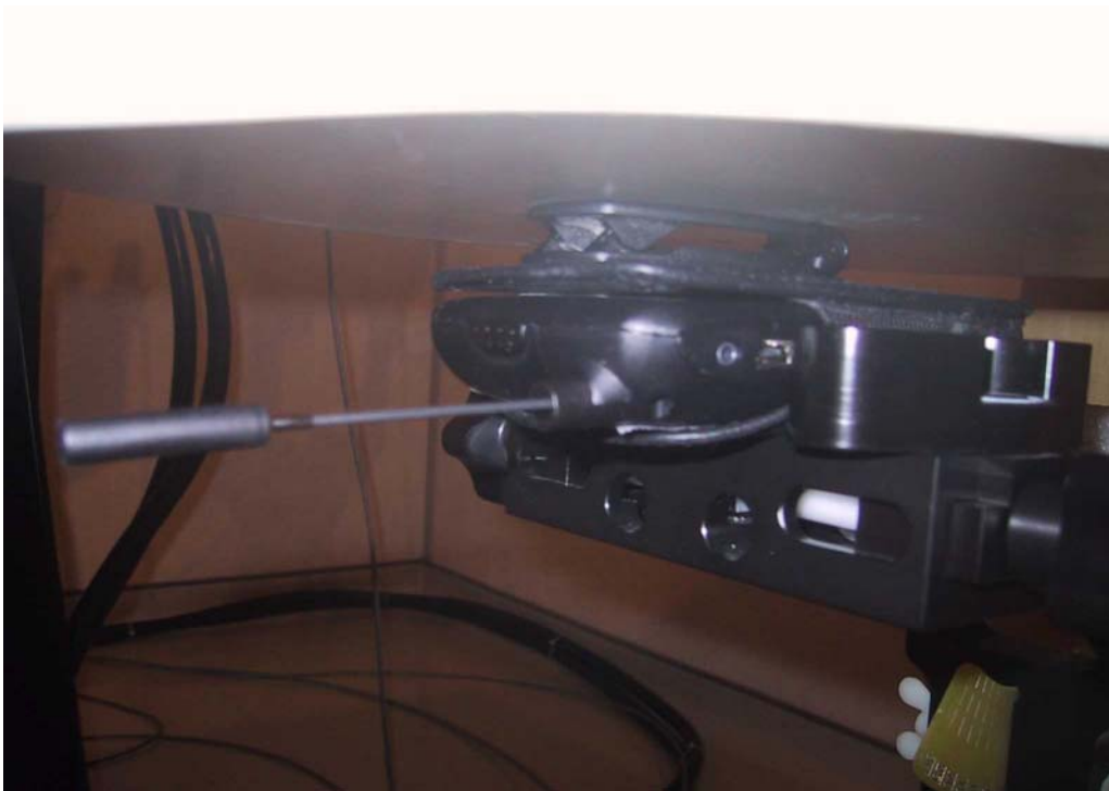
Figure E7. Body worn configuration with Leather Swivel Holster
