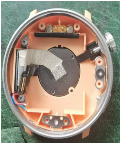
3、The horn pressing steel plate is connected to the heart rate small plate with conductive cloth
